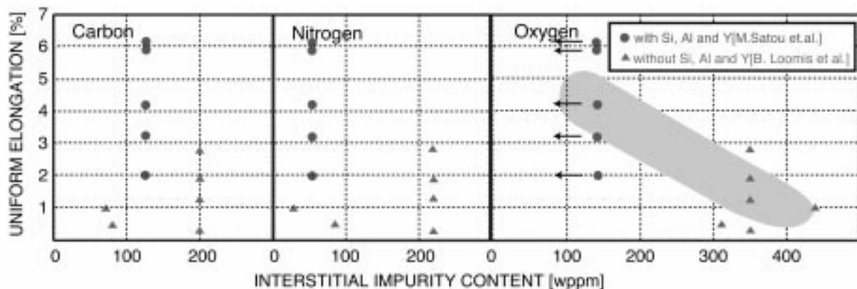
FIG. 2. Dependence of impurity content on uniform elongation of V-Ti-Cr type alloys after neutron irradiation around 400 °C up to 50dpa. Arrows indicate possible reduction of oxygen concentration in solution due to the formation of yttrium oxides.
