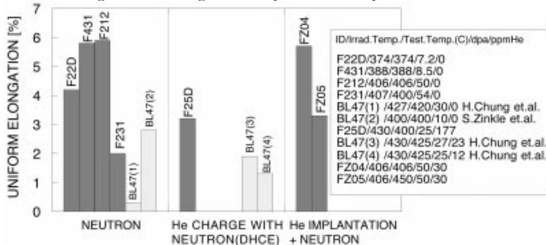
FIG. 3. Comparison of uniform elongation of V-4Cr-4Ti and modified V-Ti-Cr type alloy after neutron irradiation and He charging.
