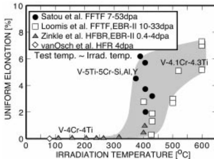
FIG. 1. Dependence on irradiation and test temperature of uniform elongation for V-4Cr-4Ti and modified V-Ti-Cr type alloy after neutron irradiation.
