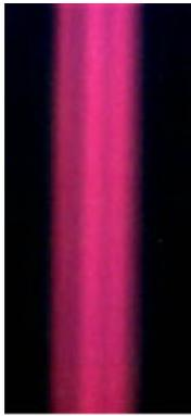
FIG.1-b 400 keV H<sup>-</sup> beamlets from 3x3 apertures in the 1 MeV beam source
