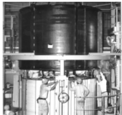
FIG. 3. A mould for VPI is being installed on the outer module
