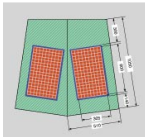
Fig.5 Split winding pack and coil casing
