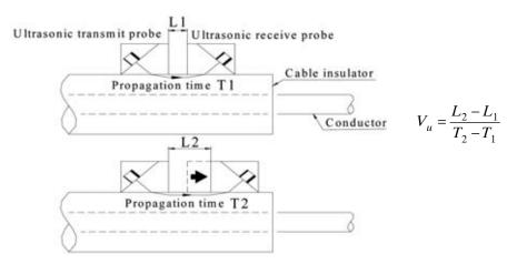
FIG. 9. Principle of ultrasonic wave propagation velocity measurement.
