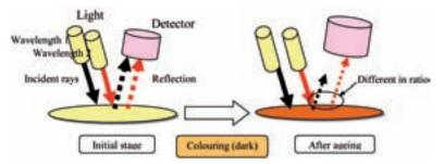
FIG. 10. Application of optical diagnosis for detecting degradation.
