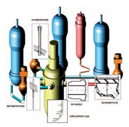
FIG. 8. Risk of stress corrosion cracking in other Inconel areas in the primary system.
