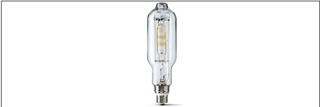
FIG. I-1. Typical example of an HID-lamp containing an inner quartz glass arc tube, a quartz glass outer envelope and an Edison fitting. (Image courtesy of Philips)
