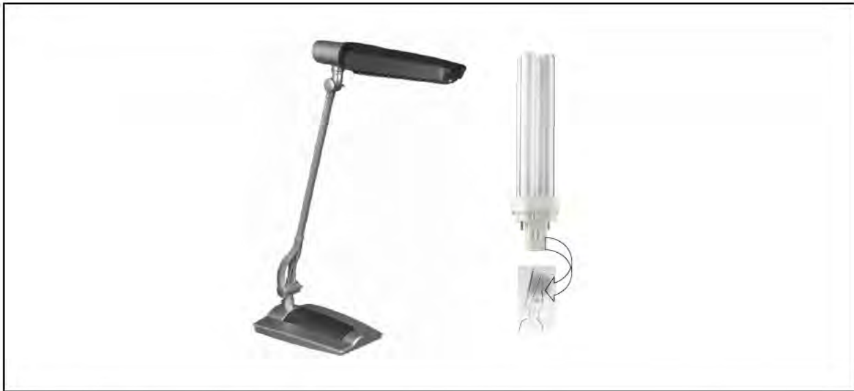
FIG. III-2. Non-integrated compact fluorescent lamp system. The image shows a desk lamp containing a non-integrated compact fluorescent lamp. The lamp on the right hand side and the glow switch that is built into the base of the lamp is shown separately underneath the lamp. (Images courtesy of Philips)
