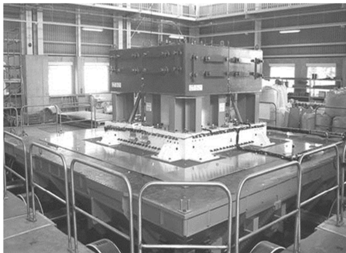
FIG. 6. Dynamic loading test showing a specimen and the shaking table.
