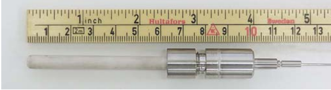
Figure 20. Prototype Fe/Fe 3 O 4 ECP reference electrode
