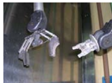
Fig. 11 – Final adjust (old tongs and fingers vs. new tongs)
