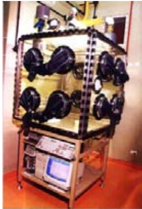
Fig. 7 – LFR Glove-Box with the HPLC system.
