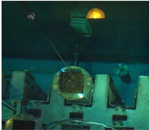
Figure 12. Exponential Experiment for Spent Fuel Assembly in PIEF Pool
