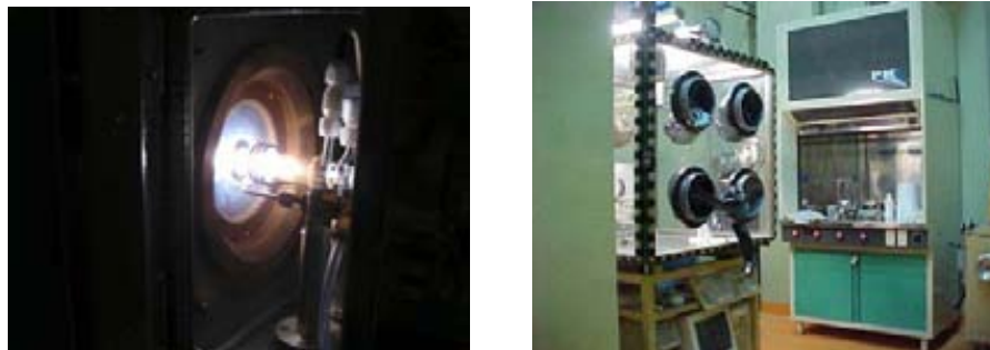
Fig. 29 and 30 – Plasma high temperature without glass-shielding protection and glove-box and fume hood in the “Controlled Area” of the hot-cell line
