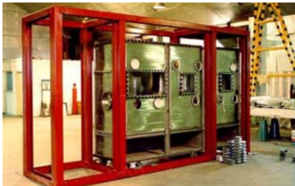
Fig. 4 – Metallic frame for the shielding and internal sealed enclosures for cells numbers 1 and 2.
