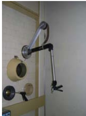
Fig. 9 – Telem manipulator “PAR” in hot-Cell N°1
