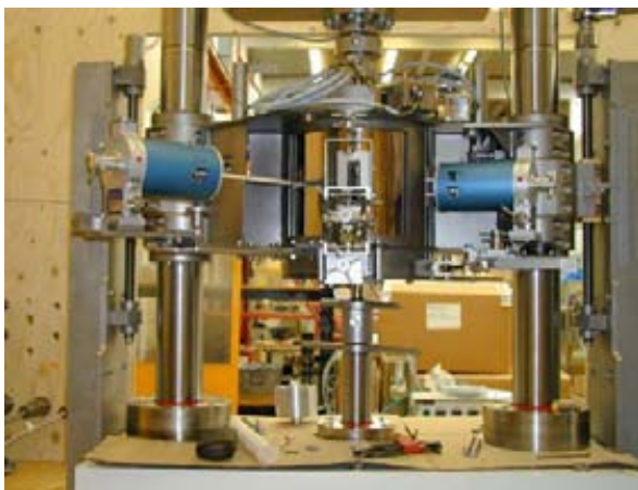
Figures 3 to 6 show ram spark erosion machining (upper left), the new optical microscope (upper right), dynamic tensile test machine (bottom left) and instrumented Charpy for sub-size specimen before installation inside the new cells (bottom right).
