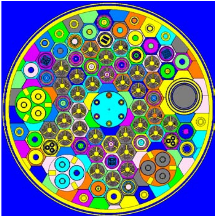
Fig. 1: Inside view of the BR2 reactor (left) and MCNP model representation of a horizontal cut 15 cm below midplane showing the hexagonal lattice with the various channels and their contents (right).
