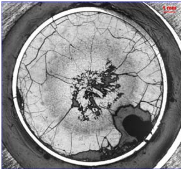
Fig-2 As polished cross section of the failed fuel near the end plug
