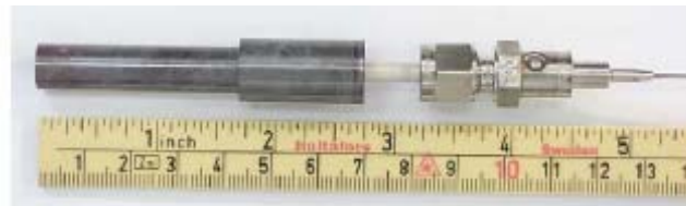
Figure 17. Halden/VTT palladium ECP reference electrode
