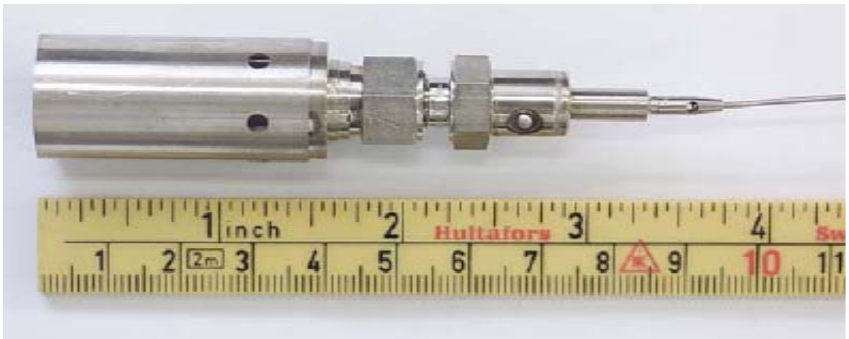
Figure 21. In-core conductivity cell
