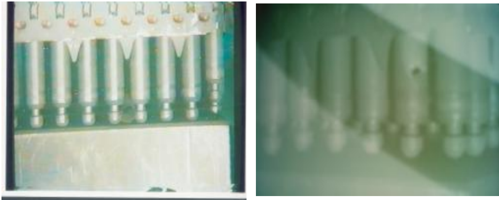
Fig. 4 Debris in the fuel assembly and fretted hole in fuel rod
