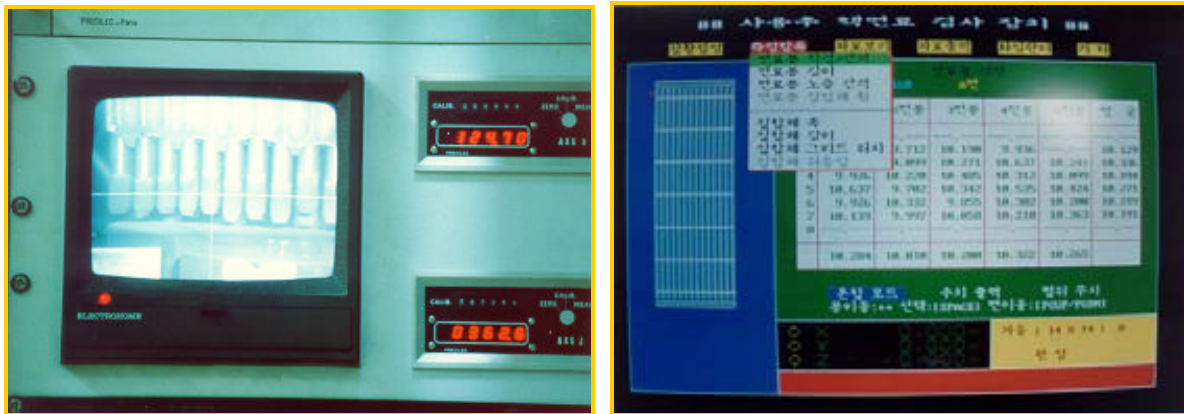
Fig. 5. Control Panel, Display Monitor & Data Acquisition System of VDIS
