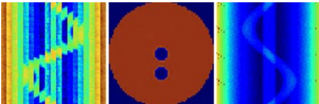
FIG. 67. Sinogram, reconstructed image and reconstructed sinogram in the noise free case.
