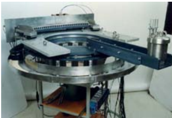
FIG. 9. 3 rd CT system developed by CEA for IFP, based on 32 shiftable detectors making it equivalent to 64 detectors per projection.
