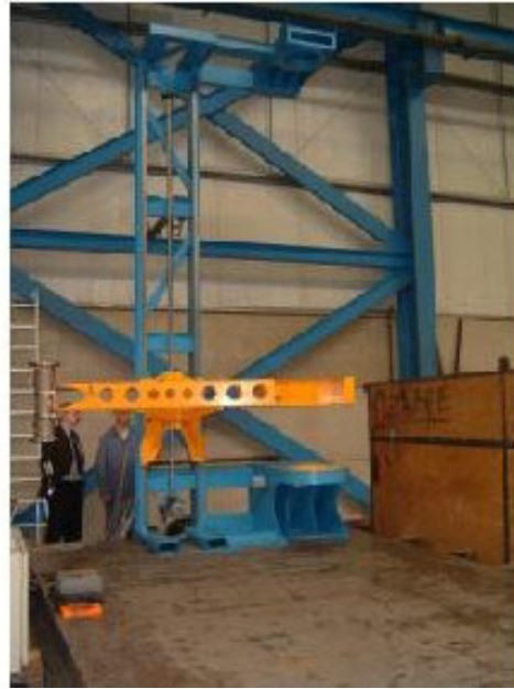
FIG. 8. X ray computed tomography set-up. A: arm; B, B': cable channel lower and upper positions; C, C': carriage lower and upper positions; D: detector bank; E: baffle; O: arm rotation vertical axis; R, R'': rotating table; R': rails; S: X-ray source; V: helicoidal screw; W: 0.6 m concrete wall.
