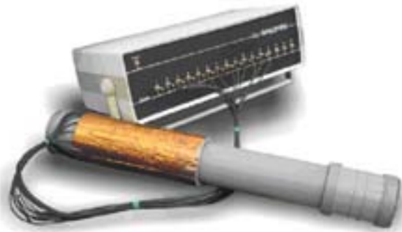
FIG. 86. ECT system ET-1 manufactured by the Warsaw University of Technology.
