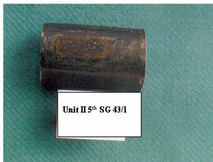
Fig. 13. Cut samples from first raw — Tubes from Paks NPP (WWER 440).
