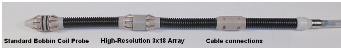
Fig. 25. Array probe with rotating magnetic field (X ® probe).
