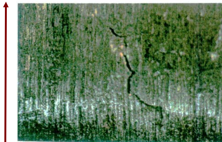
Fig. 14. Macro photographs of cracks found on Paks NPP WWER 440 steam generator tubes.
