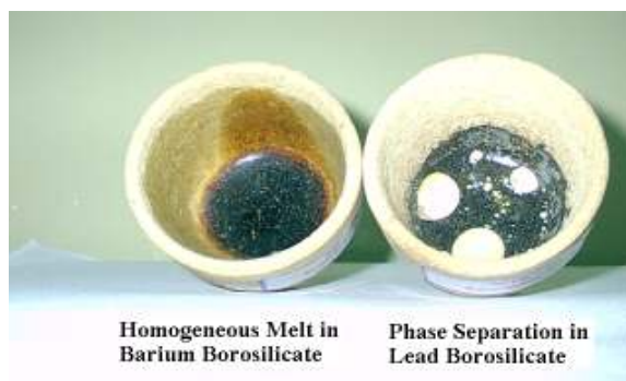
FIG. 1. Vitrified waste product based on barium borosilicate & lead borosilicate glass
