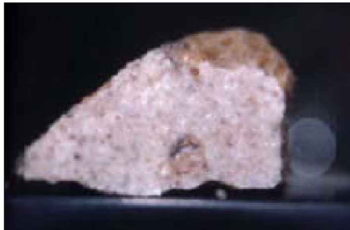
Fig. VI-40. BaSO_4 layers formed on sandstone.
