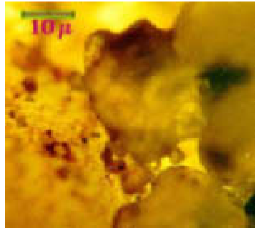
Fig. XI-64. Glueing of small particles onto big ones by polymer.
