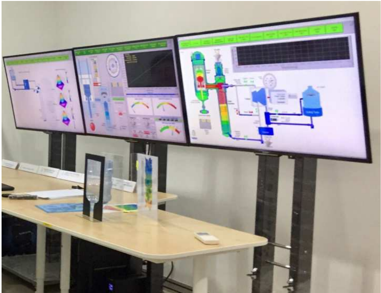
FIG. 1. Simulator with three computer screens to show the reactor control, balance of plant and cavity cooling system.
