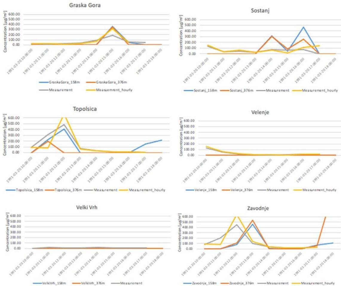
FIG. 27. Comparison of model predictions using ARTM with the measurements of SO<sub>2</sub> (µg/m<sup>3</sup>) for 20 March 1991 (10:00–17:00) at the six monitoring stations. Model results are shown for the SODAR windfield at 158 m (blue) and 376 m (orange). Measurements are shown as reported on the hour (yellow) or as averages of two half-hour measurements (grey).
