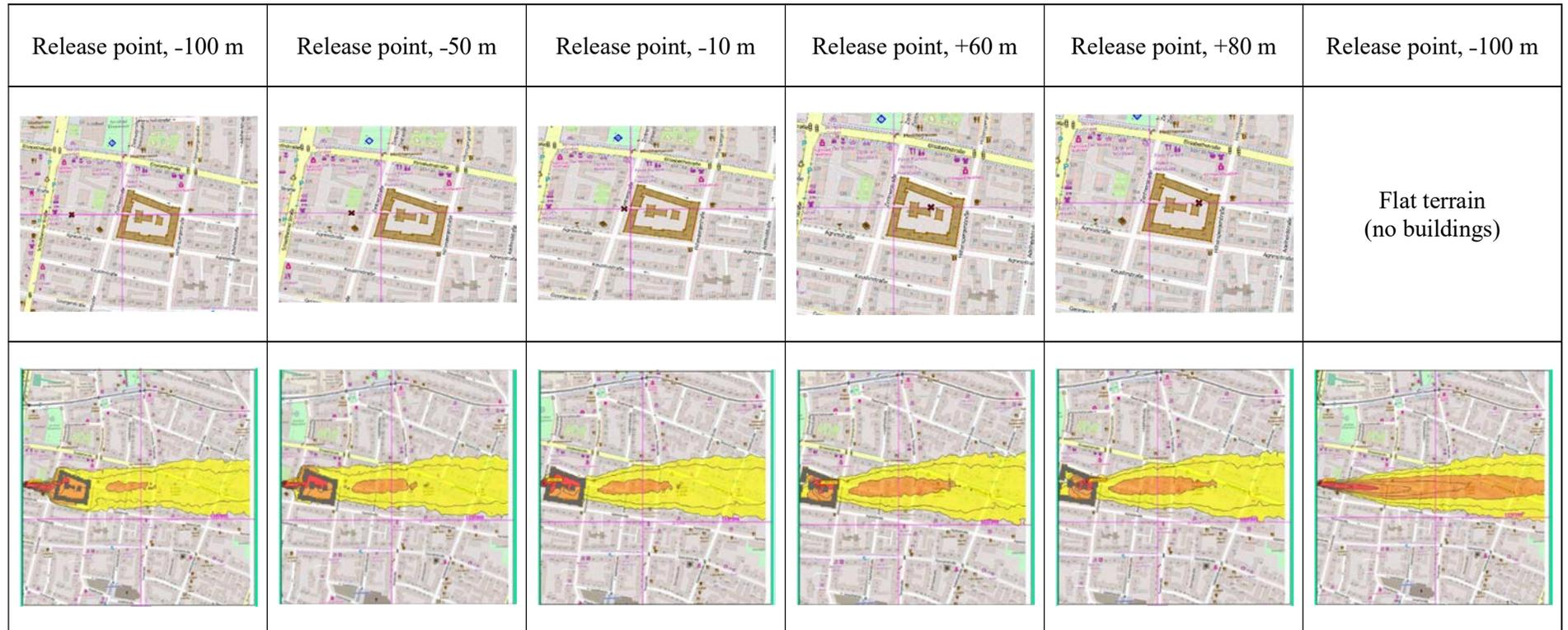
FIG. 16. Model predictions for Scenario 3 obtained with LASAIR for a 1 min continuous release, using different release points (-100 m, -50 m, -10 m, +60 m, +80 m). For the last column, the predictions assumed flat terrain (no buildings). The first row shows the dispersion point with respect to the building; the second row shows the predicted deposition after 1 h ( $Bq/m^2$ ). (Map data from OpenStreetMap <https://www.openstreetmap.org/copyright>, as used in the model LASAIR.)
