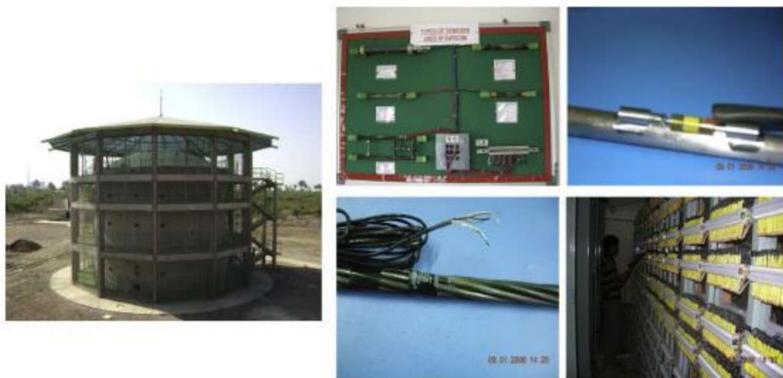
FIG. 26. BARC Containment test model at BARC-Tarapur test facility with details of embedded sensors and cable panels (courtesy of BARC, India).
