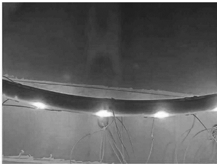
FIG. 21. Sagging study for a single channel in Argon environment (reproduced from Ref. [86] with permission courtesy of Elsevier).
