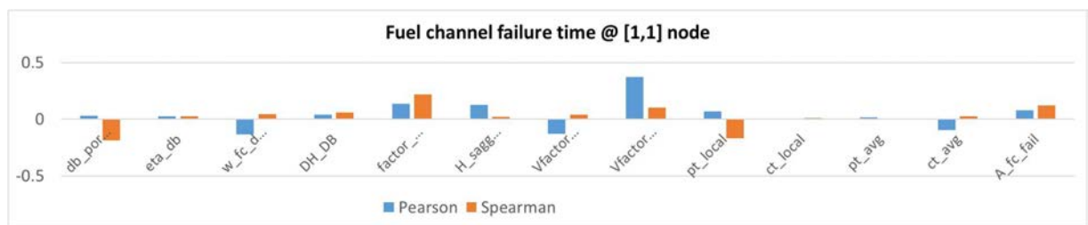
FIG. 71. Sensitivity analysis results for a fuel channel failure in the [1, 1] node.
