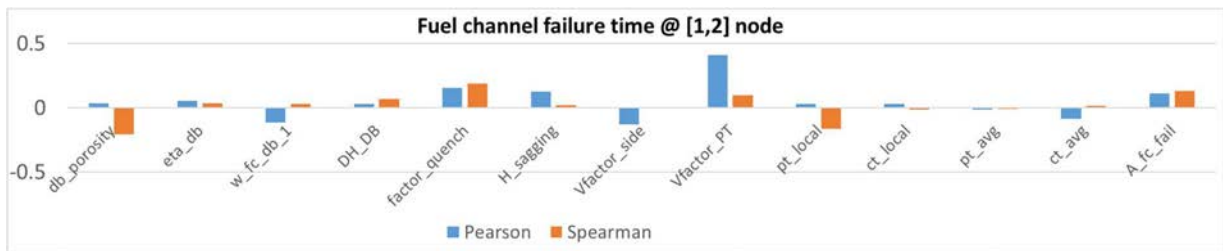
FIG. 70. Sensitivity analysis results for a fuel channel failure in the [1, 2] node.
