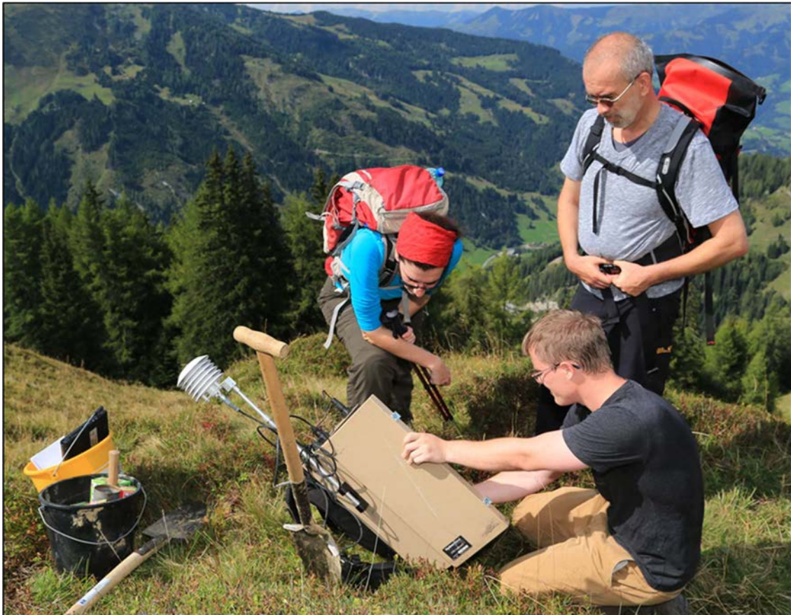
FIG. 2.1. Example of the backpack CRNS device deployed in a mountainous environment in Austria.
