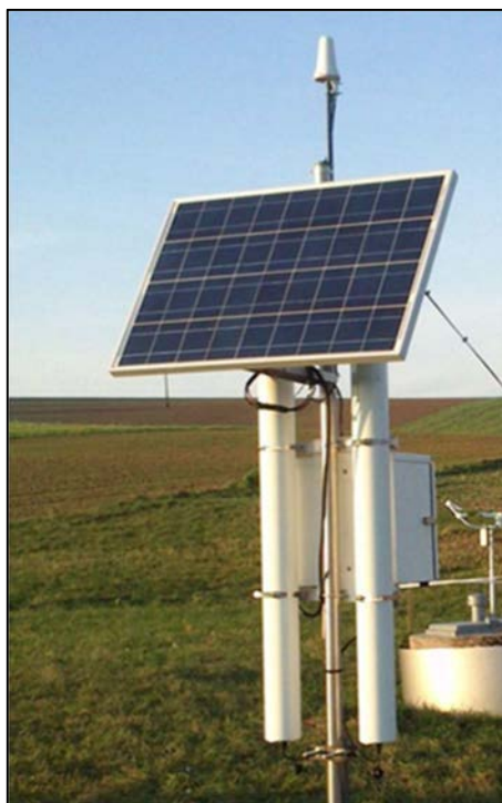
FIG. 1.1. Example of a stationary CRNS device, taken near Petzenkirchen, Austria, courtesy of the IAEA/FAO. The detectors typically accumulate neutron counts over an hour-long period.
