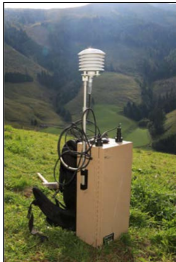
FIG. 1.3. Example of a mobile “backpack” CRNS device in Rauris Austria. The CRNS detectors are located inside the metal box and can be hand carried by a single individual. The lighter weight medium sized detectors allow for accumulated neutron counts over a period of ten to twenty minutes.
