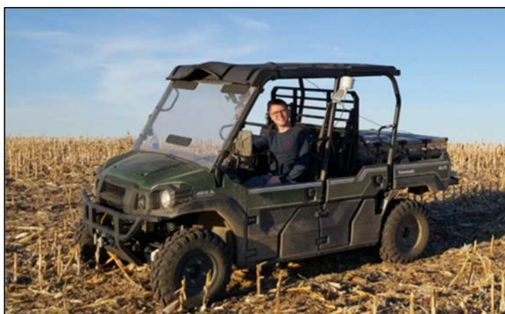
FIG. 1.2. Example of a mobile “roving” CRNS device in Nebraska USA. The boxes containing the CRNS detectors are mounted in the back of the vehicle. The larger detectors accumulate enough neutron counts over 1-minute periods to allow for mobile surveys over large areas like commercial agricultural fields typical of Nebraska.
