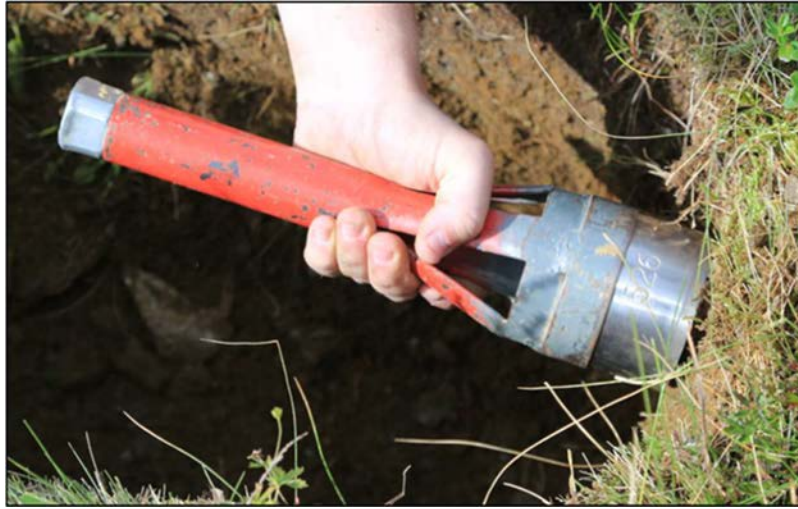
FIG. 2.2. Example of an in-situ soil sampler to determine volumetric water content and soil bulk density.
