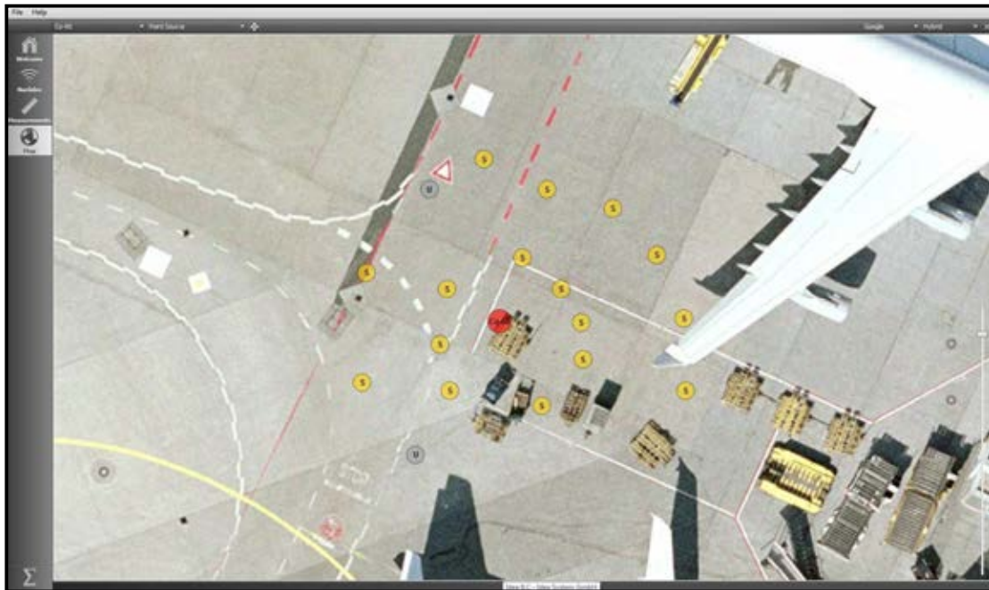
FIG. 4. Display of reconstructed point radiation source (artificial scenario at Frankfurt, Germany airport); "S" represent points contributing to source identification; "U" are points not contributing to the reconstruction of the source.
