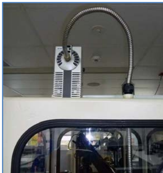
FIG. 4. Polilight® PL500 light guide and imaging system inside the glove box (left) and Polilight® PL500 unit external to the glove box (right).
