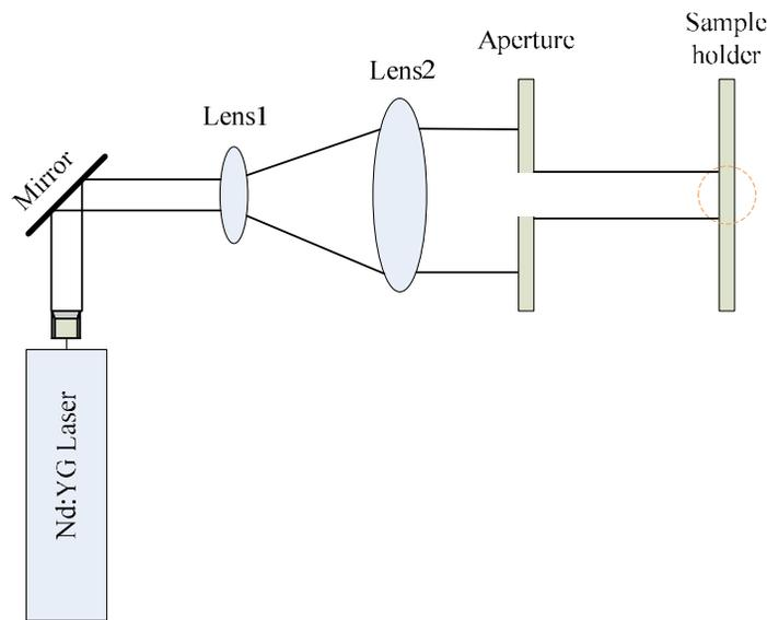
*Figure 1. Schematic diagram of pre-annealing laser exposure setup*
