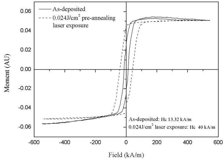
*Figure 3 Representative in-plane hysteresis loops of as-deposited (solid line) and pre-annealing pulsed laser exposed (dash line:  $0.024 \text{ J/cm}^2$ ) samples without post-annealing.*
