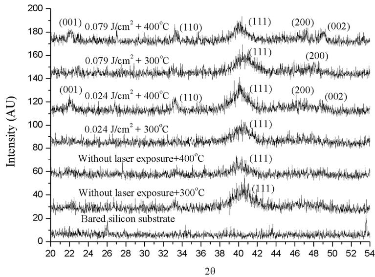
*Figure 2* XRD patterns of samples exposure at various laser energy densities and annealed at various temperatures of 300 and 400 °C.
