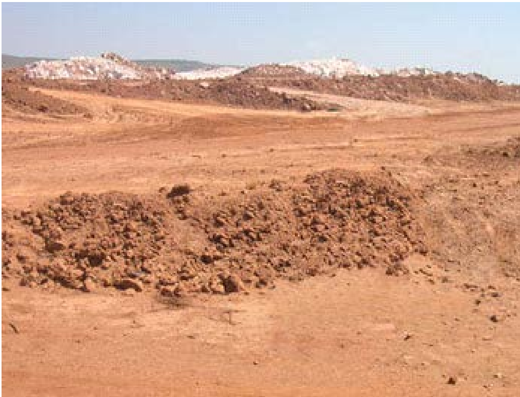
FIG. 9. Disposal of dried bauxite tailings by land spreading.
