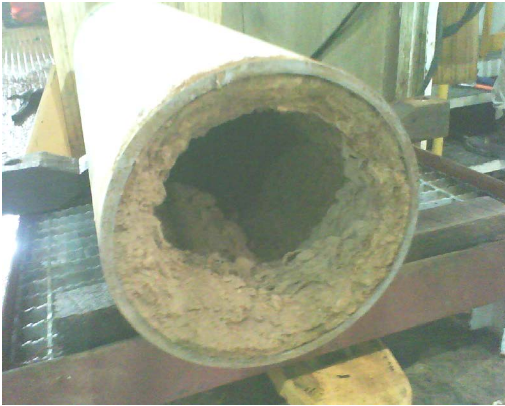
FIG. 3. Scale deposited in an oil and gas production tubular.
