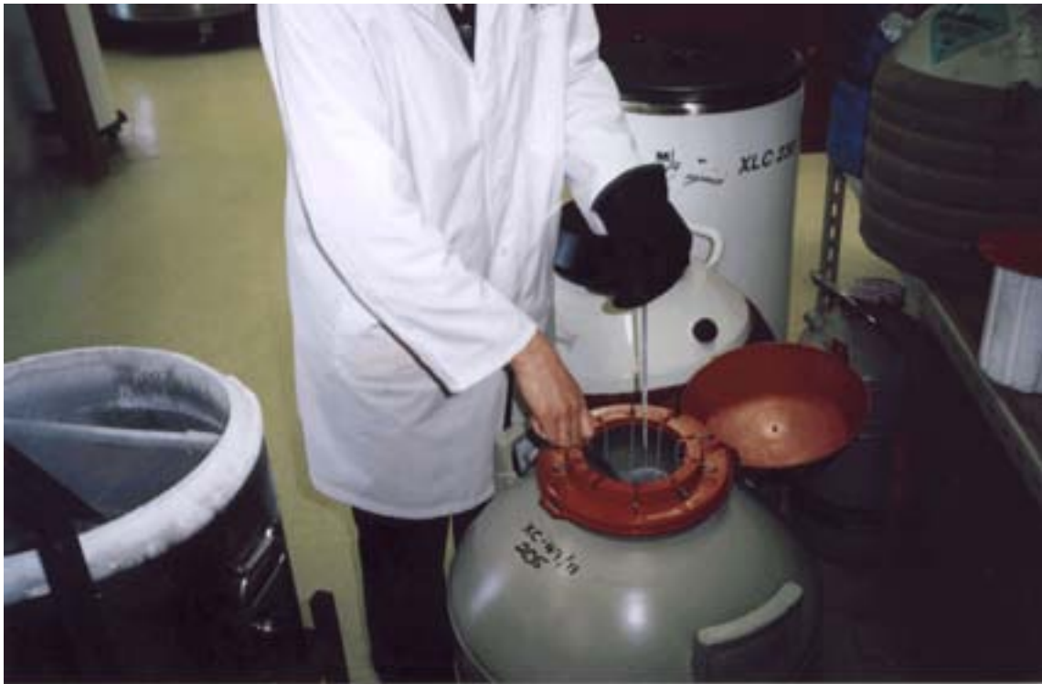
Fig. 8. When transferring frozen straws the canister should not be brought beyond the neck of the container. It should not remain there for more than ten seconds.
