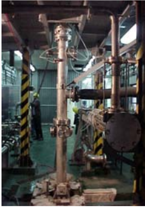
FIG. 6. Experimental Reactor's Fuel Element Test Section installed at the LPTHL.
