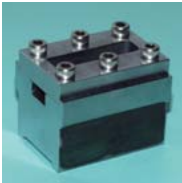
FIG. 4. Fixture for the spring characteristic test.
