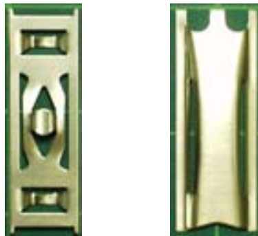
FIG. 3. KAERI devised spacer grid spring shape (Left: Opt. H; Right: Doublet-type).
