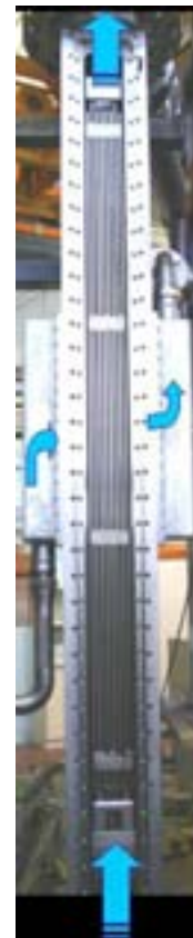
FIG. 7: Diagram of the test section MISTRAL. Front side of the test section equipped with viewport allowing laser anemometer measurements.
