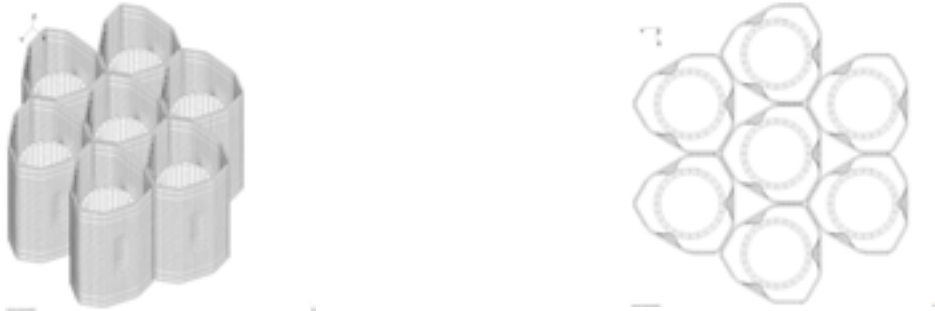
3D Fragment of the SG Model for Calculation of the Rod Model Rigidity Parameters
