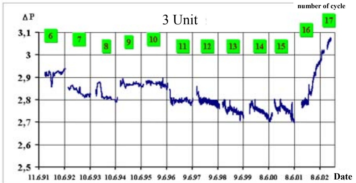
FIG. 1. Pressure drop at the 3rd unit of Paks NPP.
