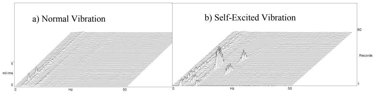
FIG. 6. Waterfall Plot of Flow Sweep Test (5 mil = 0.13 mm). Grid #4.
