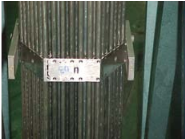
FIG. 3. Detail of one conformed sheet spacer.
