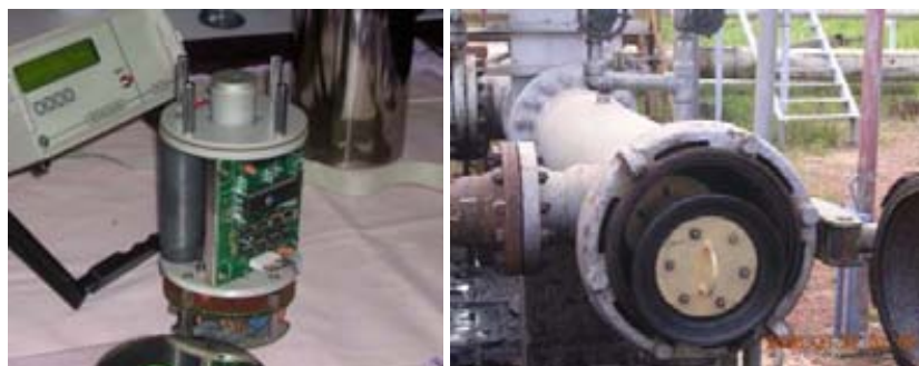
FIG. 61. Pig designed and constructed in India
