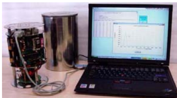
FIG. 71. Radiotracer pig data downloaded to a PC
