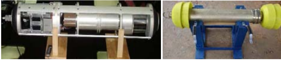
FIG. 59. Polish DN 1 pig in housing (left) and ready for using (right)
