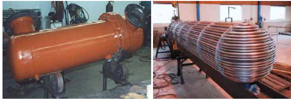
FIG. 3. A typical shell and tube type heat exchanger
