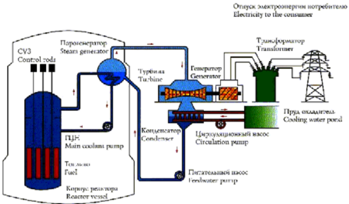
FIG. 1. Schematic diagram of NPP with WWER reactor.
