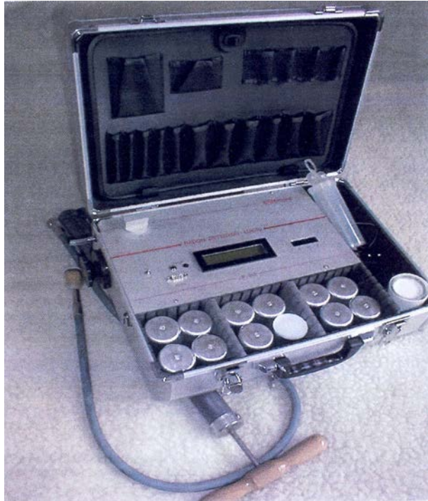
FIG. 4(a). Field radon ( ^{222}\text{Rn} ) detector LUK-3A (SSM, J.Plch, CZ). The instrument is used for analysis of radon activity concentration ( \text{kBq/m}^3 ) in soil gas. Alpha radiation of radon is detected by means of Lucas cells.
