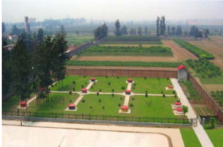
FIG. 7. Stationary calibration pads used in the calibration of portable gamma ray surveying instruments at the Airborne Survey and Remote Sensing Centre of Nuclear Industry (ARCN), China [52].
