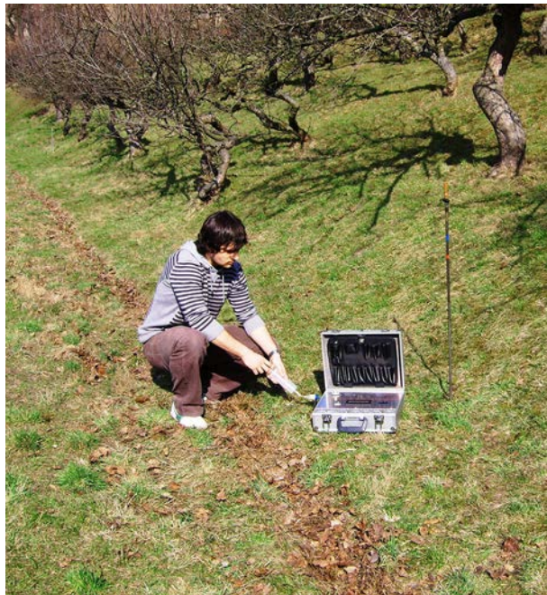
FIG. 4(b). Field use of LUK-3A; the operator is transferring soil gas into the detector.
