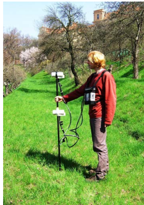
FIG. 6. Magnetometer and GSM-19 gradiometer and the Overhauser system (GEM Systems, Inc.). This instrument measures the total magnetic field and vertical gradient of the magnetic field with a sensitivity of 0.01 nT.
