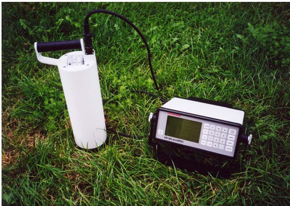
FIG. 3(a). Portable gamma ray spectrometer GR-320 (Exploranium). The spectrometer is equipped with a 350 cm 3 scintillation NaI(Tl) detector and used for radiometric prospecting, assays of K, U and Th in rocks, monitoring of environmental radiation and identification of radionuclides.
