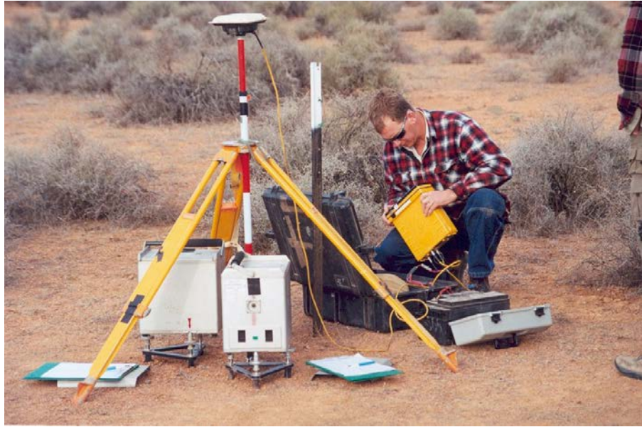
FIG. 5. Modern gravity surveys require highly accurate GPS systems to resolve ever smaller anomalies. This survey from Australia shows two gravity meters under a GPS controlled base station.
