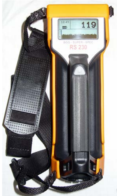
FIG. 2. A typical lightweight portable gamma ray differential spectrometer equipped with a BGO scintillation crystal and auto-stabilization on naturally occurring radioactivity peaks (Radiation Solutions, Inc.).
