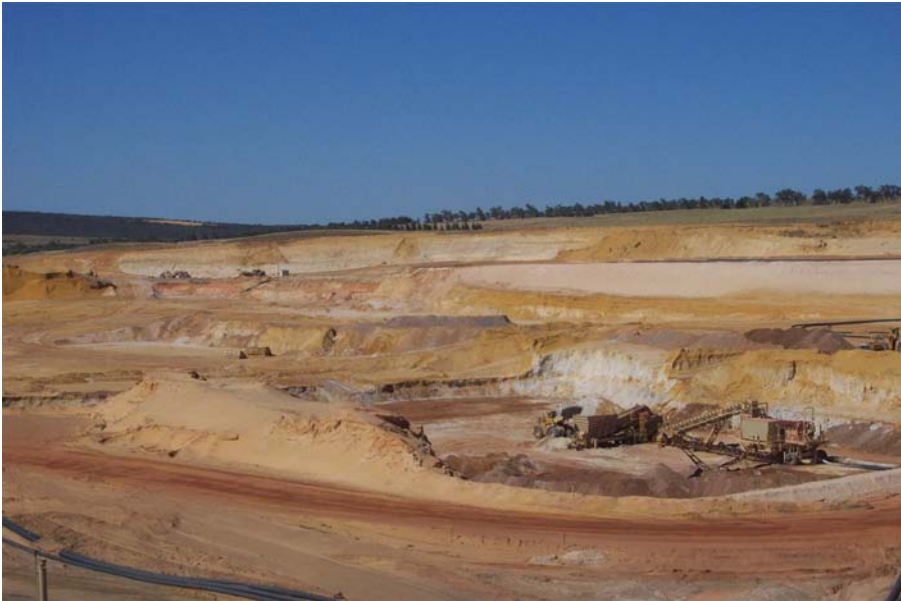
FIG. 8. Dry mining operation, showing pre-concentration operations in the foreground.
