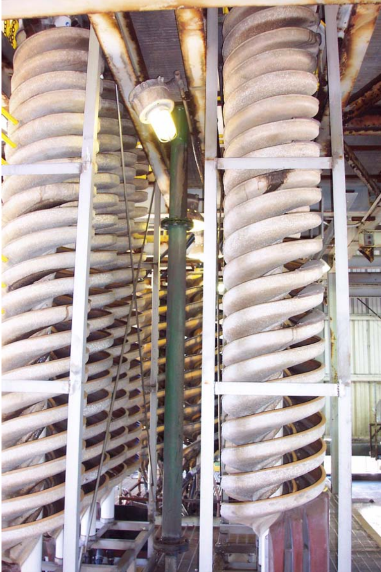
FIG. 11. Groups of spirals used in the primary separation process.
