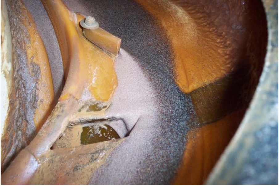
FIG. 12. Detailed view of a spiral used in the primary separation process.
