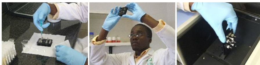
FIG. 25. Procedure for filling the cell. The cell should be filled using a 1 mL syringe, bubbles should be checked for by holding the cell up to a light, and the cell should be placed in the sample chamber of the FTIR instrument.
