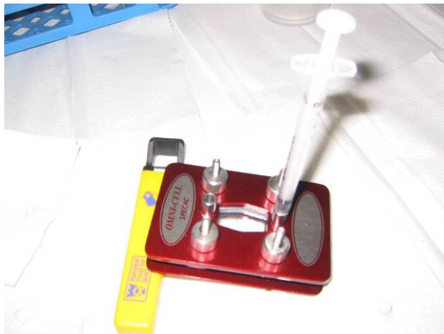
FIG. 24. FTIR cell with a 1 mL syringe in the filling port. The cell is raised at one end by propping on any suitable object, e.g. a pencil.
