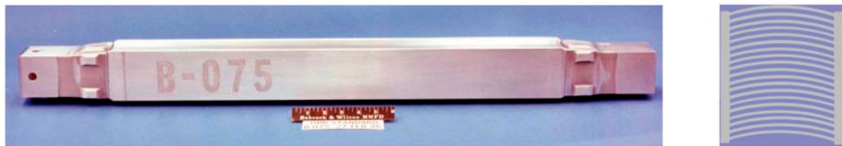
FIG. II.2. ORR LEU fuel assembly and fuel assembly cross-section.
