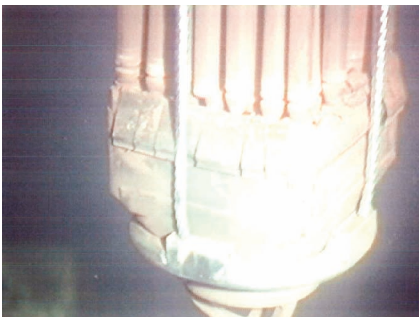
FIG. 6. Example 1: Bottom of BWR assembly fitted with securing ring and four wires (two shown) which run the full length of the assembly and are secured to an additional tie plate at the top of the assembly.
