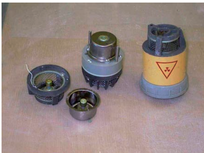
FIG. 6. Partially dismantled smoke detector containing ^{239}\text{Pu} (Soviet design).
