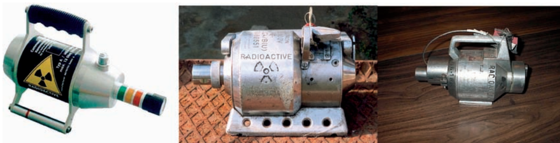
FIG. 5. Examples of gamma radiography afterloaders containing ^{192}\text{Ir} or ^{137}\text{Cs} sources.
