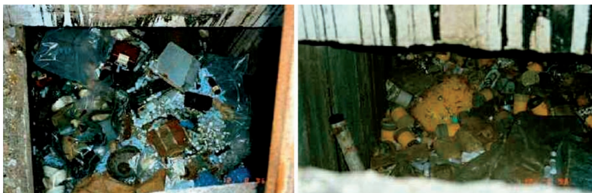
FIG. 1. Storage of historical miscellaneous waste, including disused sealed radioactive sources [7].
