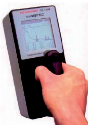
FIG. 24. Typical hand-held instrument used for location and identification of disused sealed radioactive sources.
