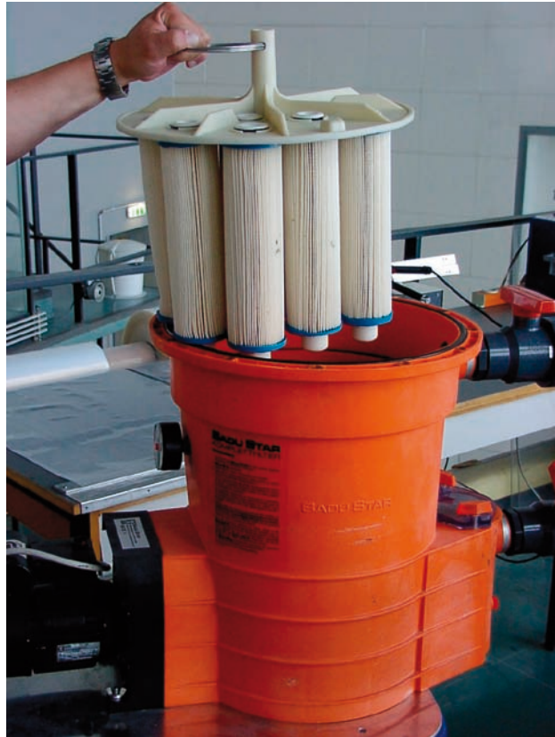
FIG. 4. Tank cleaning pump with integrated filters.
