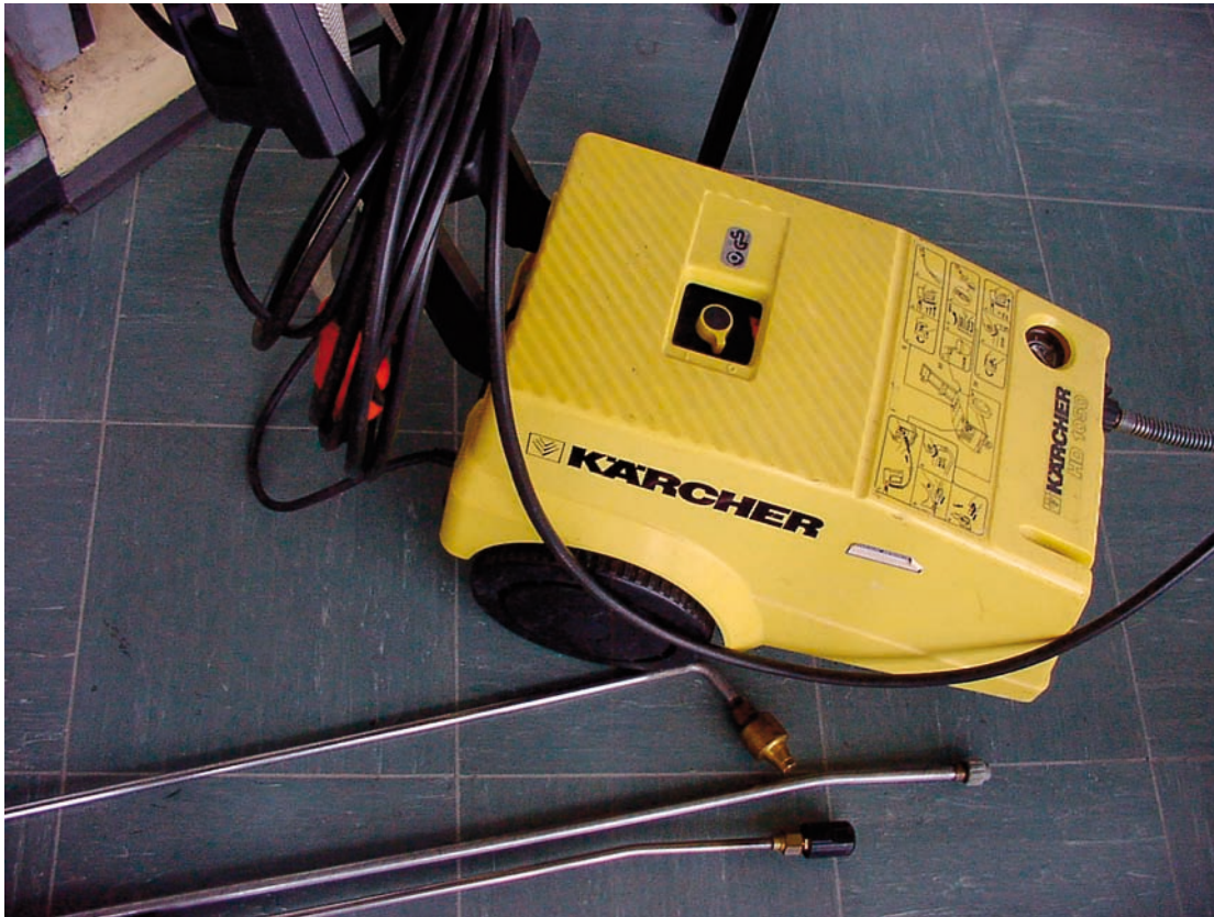
FIG. 5. Underwater jet to remove deposits.
