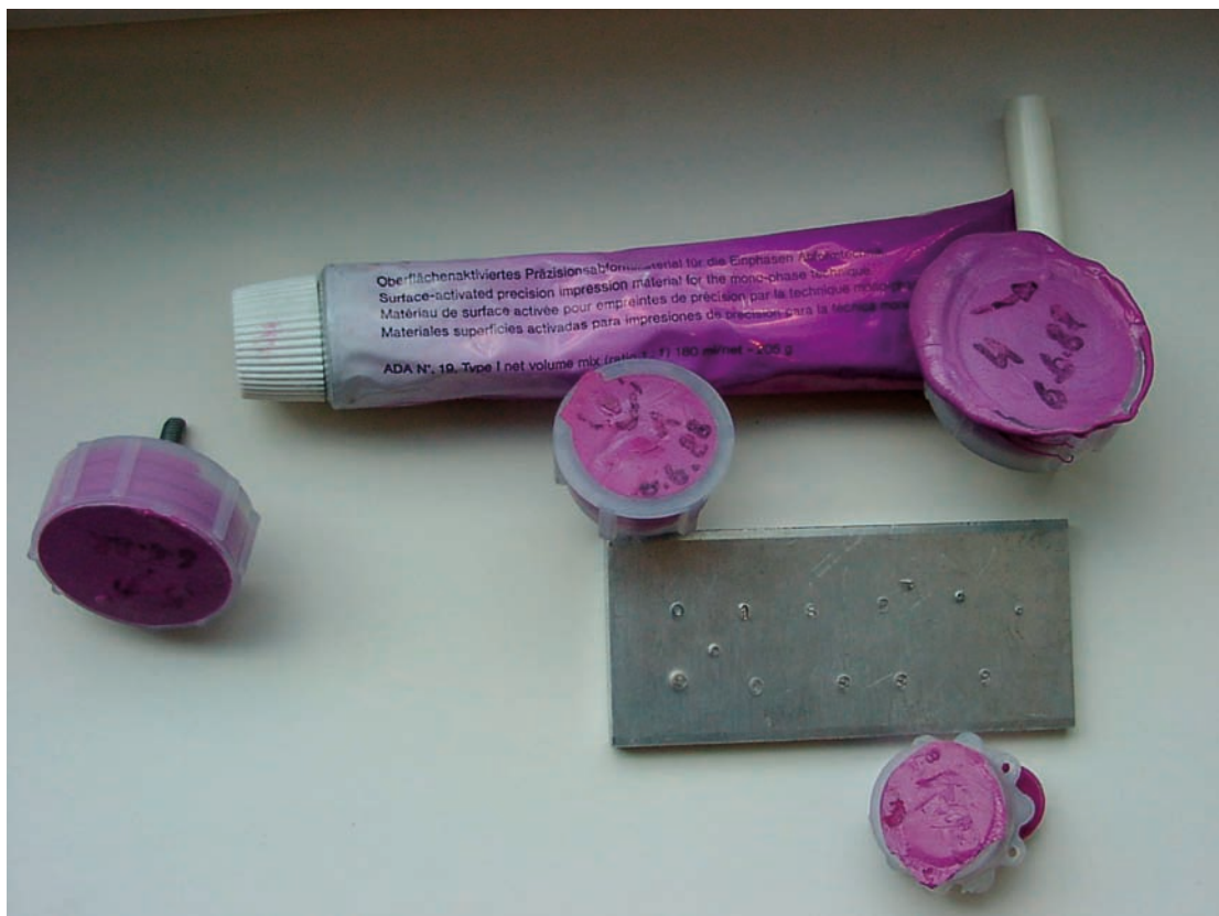
FIG. 3. Replica material to determine the dimension of a corrosion spot.
