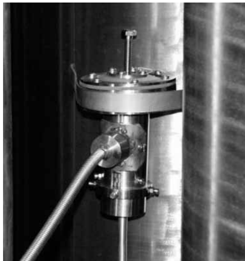
FIG. 6. Acoustic leakage detector with waveguide.
