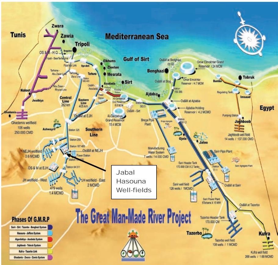
FIG. 1. Configuration of well-fields and pipelines of the GMRP, showing the Jabal Hasousa Well-fields [1].
