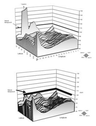
FIG. 2. Results from the final dose rate survey of the area (a) before and (b) after the surface decontamination.
