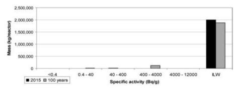
FIG. 5. Typical Magnox reactor graphite inventory.
