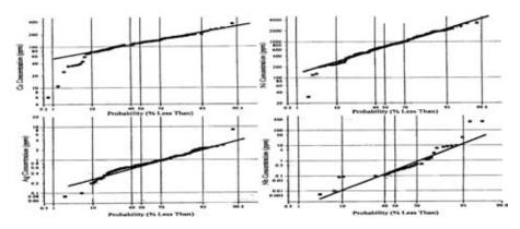
FIG. 2. Log-probability plots showing concentrations of cobalt, nickel, silver and niobium in Magnox reactor steels.
