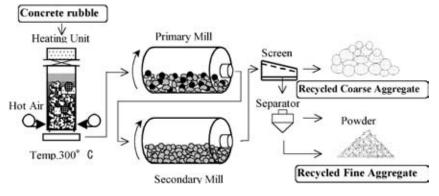
FIG. 1. Heating and grinding method.
