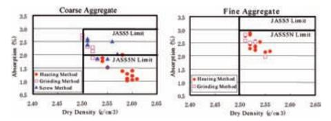
FIG. 3. Relationship between density and absorption of recycled aggregate.
