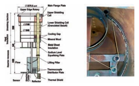
FIG. 3. Schematic view of KNK reactor rotary lid and 'mock up' for dry cutting test with a diamond wire rope.
