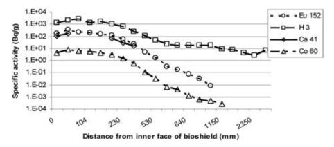
FIG. 3. Data from a core through a Magnox steel pressure vessel bioshield (note that the x axis is not linear to allow detail at the inner face to be more readily seen).
