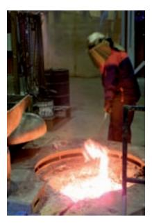
FIG. 5. Removal of slag.
