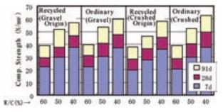
FIG. 4. Compression strength of recycled aggregate concrete and ordinary concrete.
