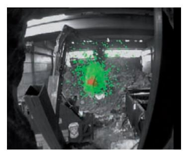
FIG. 3. The moment of removal of a high level radiation source by a robot. The image was obtained with the gamma camera.
