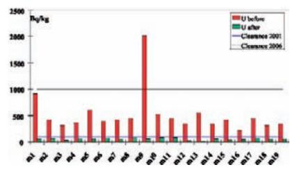
FIG. 3. Results of the melt decontamination process for uranium in steel.
