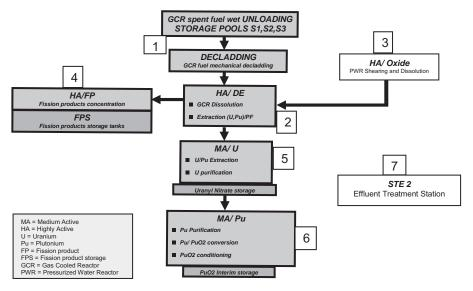
FIG. 1. UP2 400 reprocessing plant modules.
