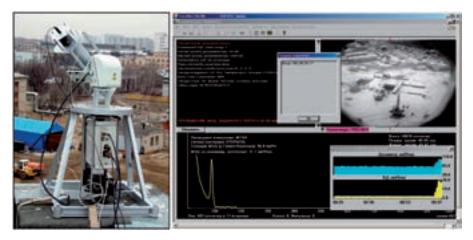
FIG. 4. The image on the gamma locator display during operations at repository No. 4 with the shadow shielding erected.
