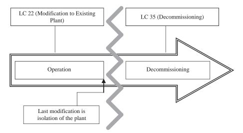
FIG. 2. Proposed use of licence conditions for a decommissioning project confined to deplanting and demolition.
