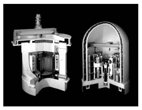
FIG. 1. Comparison between a Magnox reactor and a PWR (both pictures to approximately the same scale) (acknowledgement: www.scienceandsociety.co.uk).
