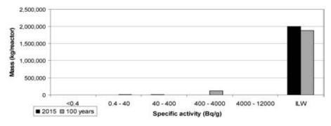
FIG. 6. Typical Magnox reactor concrete inventory.
