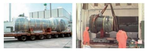
FIG. 1. Transportation and treatment of the MZFR steam generators.
