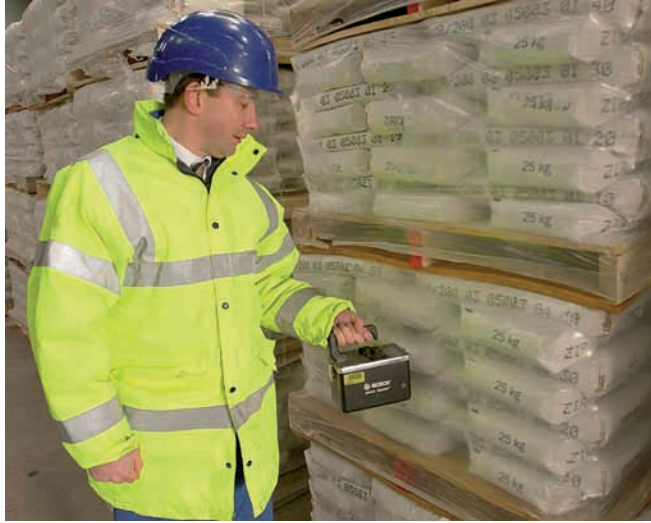
FIG. 3. Measurement of gamma dose rates near bulk quantities of zircon (courtesy UK Health Protection Agency: Centre for Radiation, Chemical and Environmental Hazards, Radiation Protection Division).
