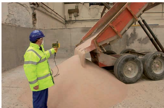
FIG. 5. Measurement of dust levels with a real time dust monitor (courtesy UK Health Protection Agency: Centre for Radiation, Chemical and Environmental Hazards, Radiation Protection Division).
