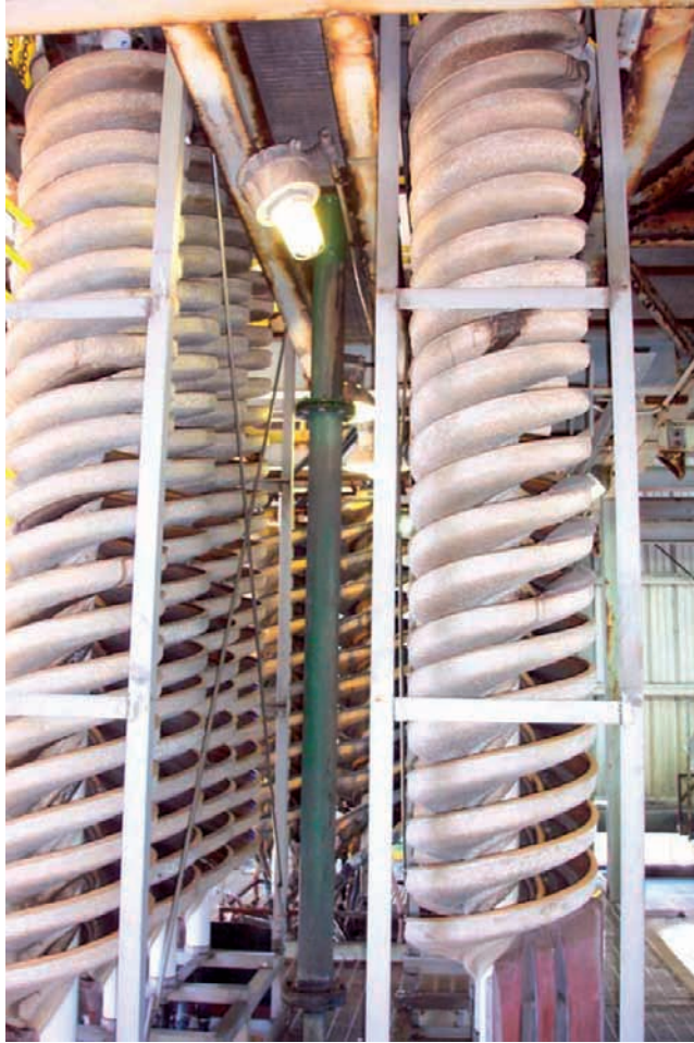
FIG. I-2. Groups of spirals used in the primary separation process.
