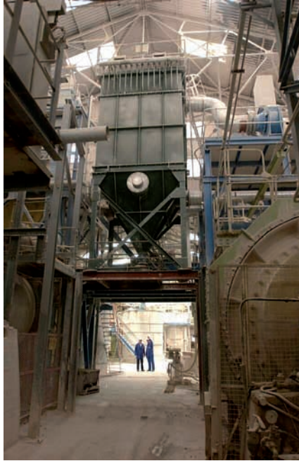
FIG. 6. Dust extraction system in a zircon milling plant (courtesy UK Health Protection Agency: Centre for Radiation, Chemical and Environmental Hazards, Radiation Protection Division).
