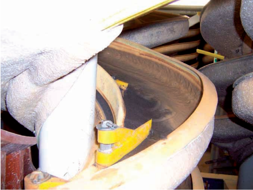
FIG. I-3. Detailed view of a spiral used in the primary separation process.
