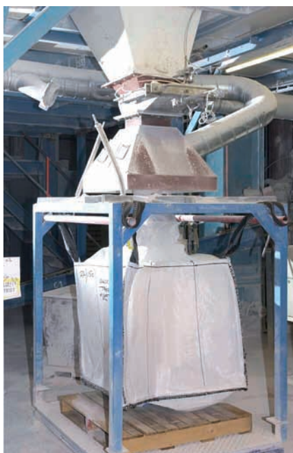
FIG. 9. Dust extraction system on bagging equipment (courtesy UK Health Protection Agency: Centre for Radiation, Chemical and Environmental Hazards, Radiation Protection Division).
