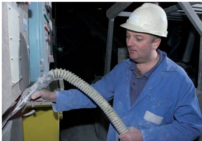
FIG. 7. Cleaning operations with a vacuum system (courtesy UK Health Protection Agency: Centre for Radiation, Chemical and Environmental Hazards, Radiation Protection Division).
