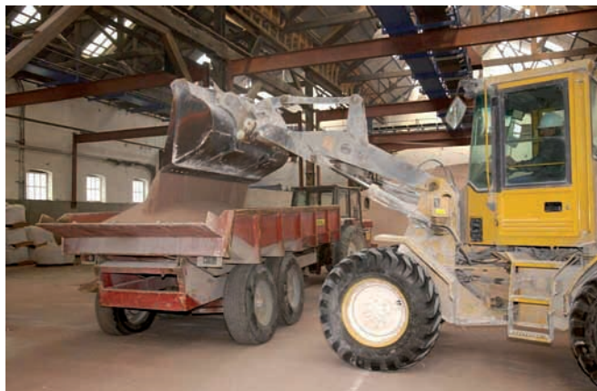
FIG. 4. Handling of zircon sand and the potential for airborne dust generation (courtesy UK Health Protection Agency: Centre for Radiation, Chemical and Environmental Hazards, Radiation Protection Division).
