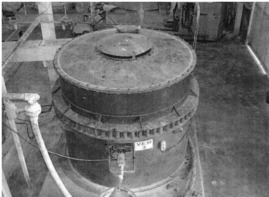
FIG. 8. Vibro-energy mill for the production of micronized zircon.
