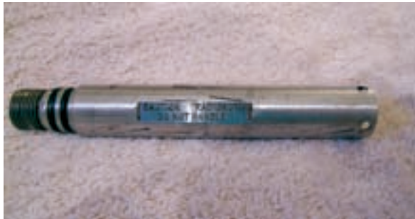
FIG. 39. Typical ^{241}\text{Am}/\text{Be} neutron oil well logging source.
