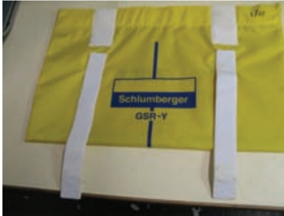
FIG. 133. Calibration blanket for a natural gamma oil well logging detector (photograph: Schlumberger).
