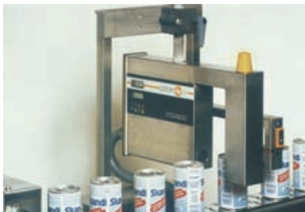
FIG. 71. Typical ^{241}\text{Am} fill-level gauge mounted on a filling line (photograph: NRC).
