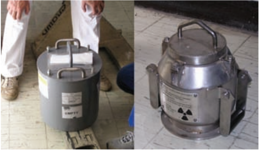
FIG. 142. High energy gamma source package showing outer package and inner shielded pot.
