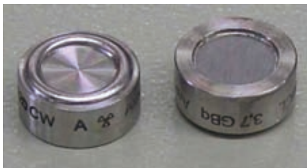
FIG. 126. Typical low energy gamma medium diameter analytical disc source showing a beryllium window and welded ends (photograph: QSA-Global).
