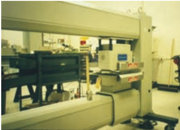
FIG. 74. Beta gauge in place on a web processing mill (photograph: NRC).
