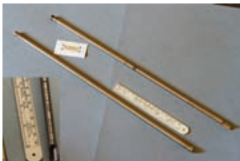
FIG. 102. Typical industrial sterilization source; the inset shows cobalt metal pellets (photograph: REVISS). Approximate dimensions: 11 mm diameter \times 450 mm length; typical activity when new: 444 TBq (12 kCi) ^{60}\text{Co} .
