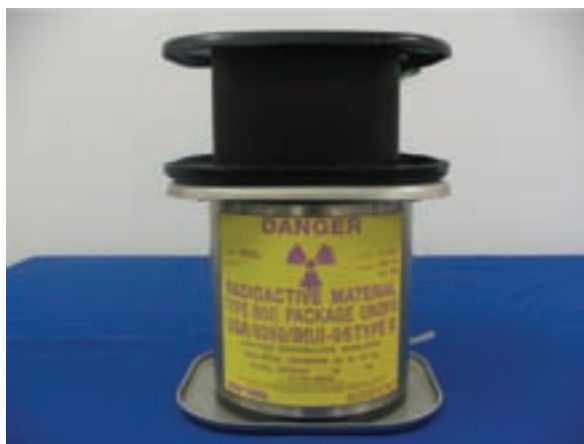
FIG. 138. Source changer in transport configuration (photograph: QSA).
