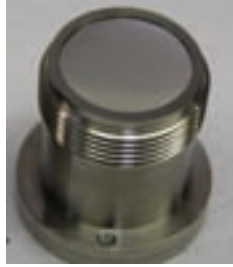
FIG. 117. ^{85}\text{Kr} beta source showing a window end (photograph: QSA-Global).
