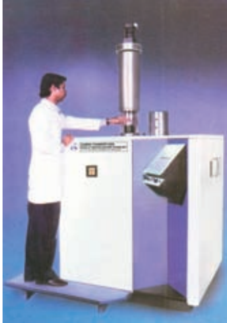
FIG. 22. Typical sample irradiator (photograph: BRIT).
