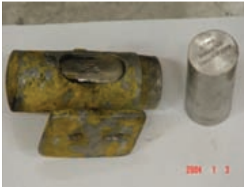
FIG. 112. Historic ^{226}\text{Ra} gamma gauging source and source holder.
