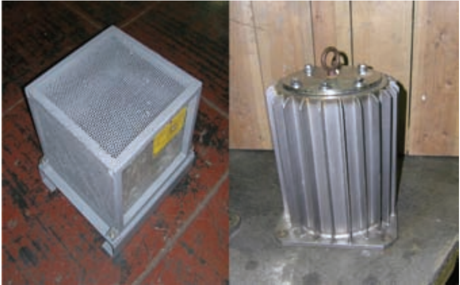
FIG. 144. High energy gamma source package showing outer package and inner shielded pot (photograph: MAYAK P.A.).
