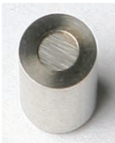
FIG. 127. Typical low energy gamma small diameter disc source showing a beryllium window (photograph: IPL).
