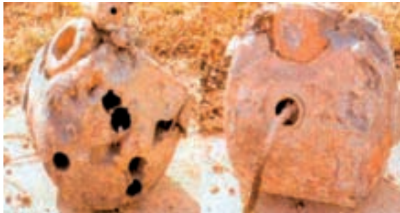
FIG. 15. Damaged ^{60}\text{Co} or ^{137}\text{Cs} teletherapy heads.
