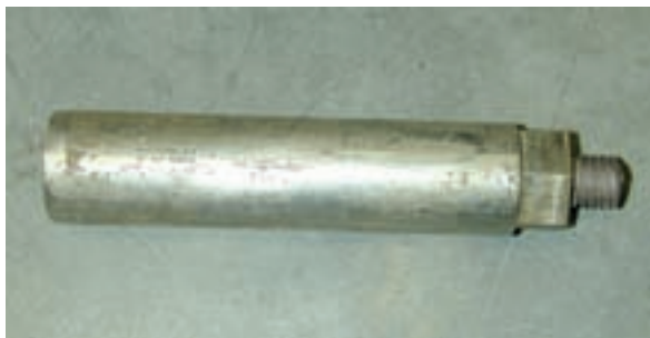
FIG. 40. Typical ^{238}\text{Pu}/\text{Be} neutron oil well logging source.
