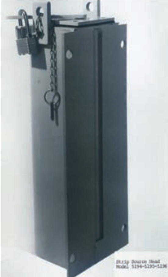
FIG. 68. Typical line source container (photograph: NRC).
