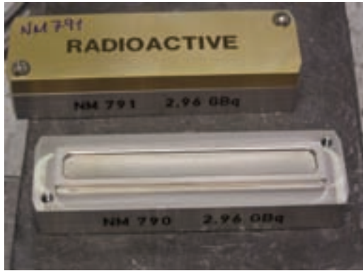
FIG. 118. ^{85}\text{Kr} beta sources with a protective brass window cover, attached and removed (photograph: QSA-Global).
