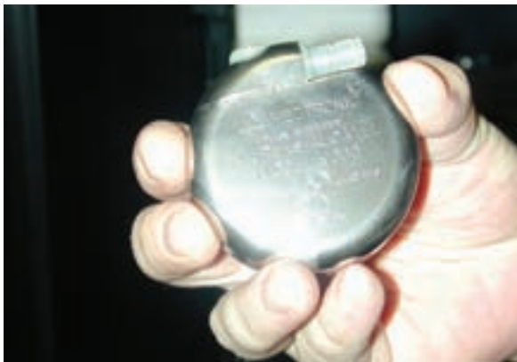
FIG. 33. Radioisotope thermoelectric generator powered heart pacemaker.
