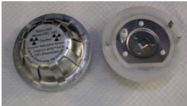
FIG. 98. Typical ion chamber containing the radioactive component from a domestic smoke detector (photograph: QSA-Global).
