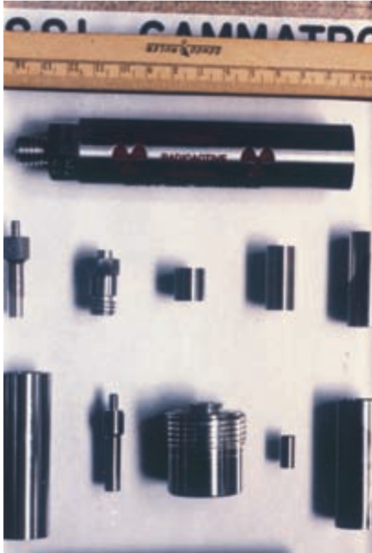
FIG. 114. A selection of ^{241}\text{Am}/\text{Be} and ^{137}\text{Cs} oil well logging sources (photograph: NRC).
