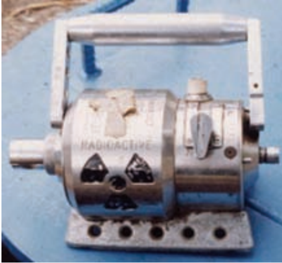
FIG. 49. Typical modern portable gamma radiography projector (photograph: NE-Seibersdorf).
