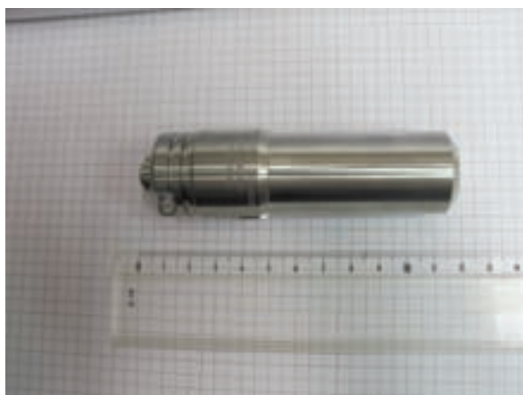
FIG. 34. Typical ^{137}\text{Cs} oil well logging source bull plug (photograph: Schlumberger).
