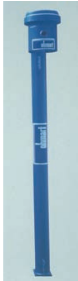
FIG. 69. Typical line source container (photograph: NRC).
