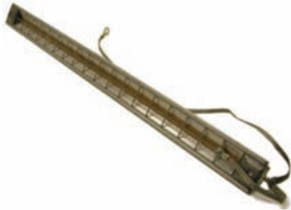
FIG. 89. Typical static eliminator bar (photograph: Oak Ridge Associated Universities).
