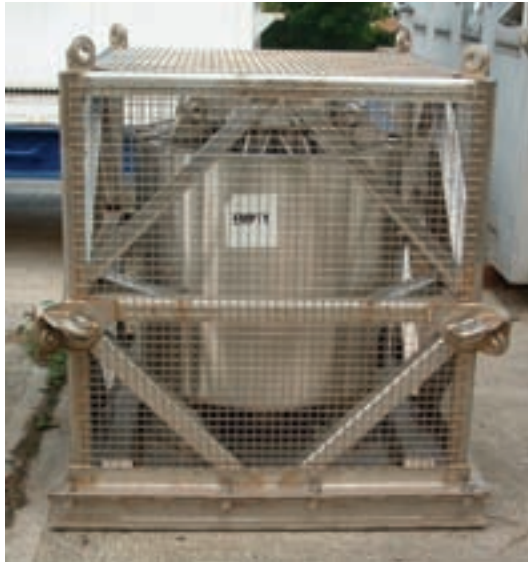
FIG. 135. High activity gamma source container enclosed in a cage to prevent contact with its hot surfaces (photograph: REVISS).
