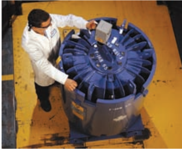
FIG. 136. Checking surface dose rates before dispatch of a high activity gamma source container (photograph: MDS Nordion).
