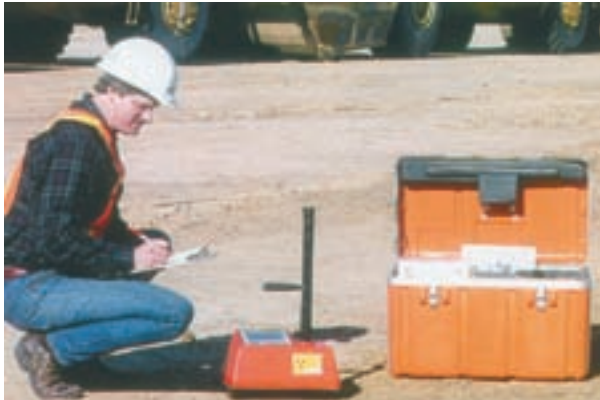
FIG. 78. Typical soil moisture and density gauge, shown with a carrying case (photograph: CPN International).
