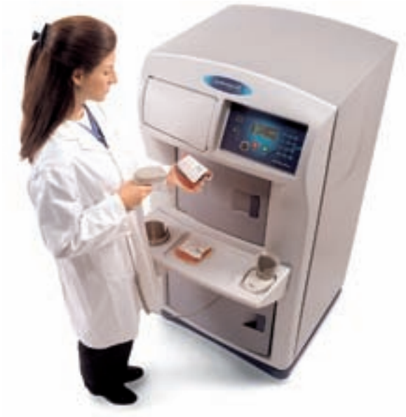
FIG. 16. Typical blood irradiator (photograph: MDS Nordion).
