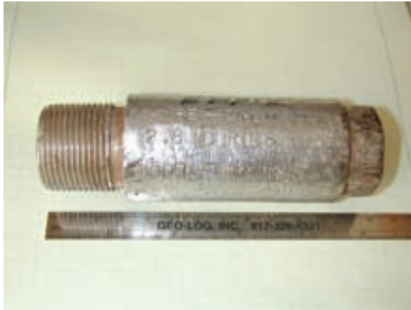
FIG. 37. Typical ^{241}\text{Am}/\text{Be} neutron oil well logging source — damaged in routine use.
