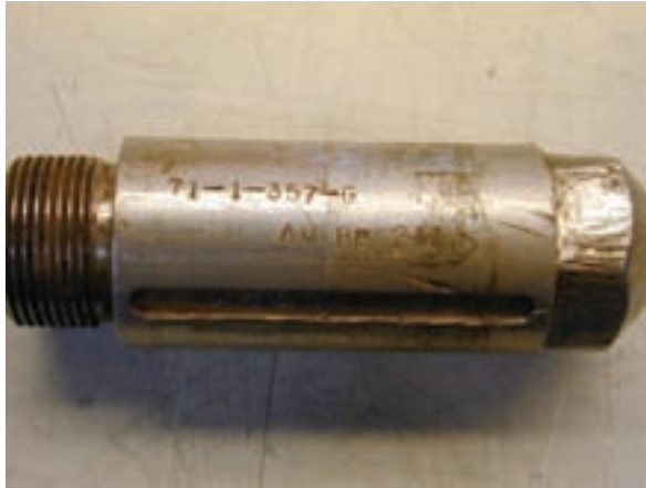
FIG. 38. Typical ^{241}\text{Am}/\text{Be} neutron oil well logging source.
