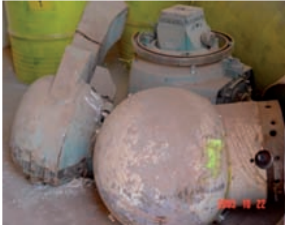
FIG. 14. Old ^{60}\text{Co} teletherapy heads.
