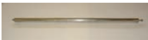
FIG. 103. Typical industrial sterilization source (photograph: REVISS). Approximate dimensions: 35 mm diameter \times 720 mm length; typical activity when new: 1.85 PBq (50 kCi) ^{60}\text{Co} .
