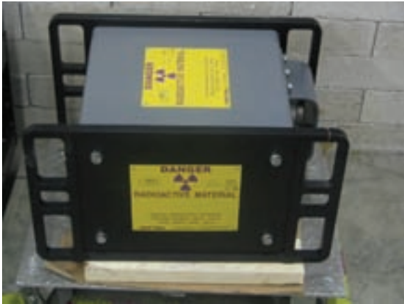
FIG. 54. Typical modern semi-portable ^{60}\text{Co} gamma radiography device (photograph: QSA-GLOBAL).
