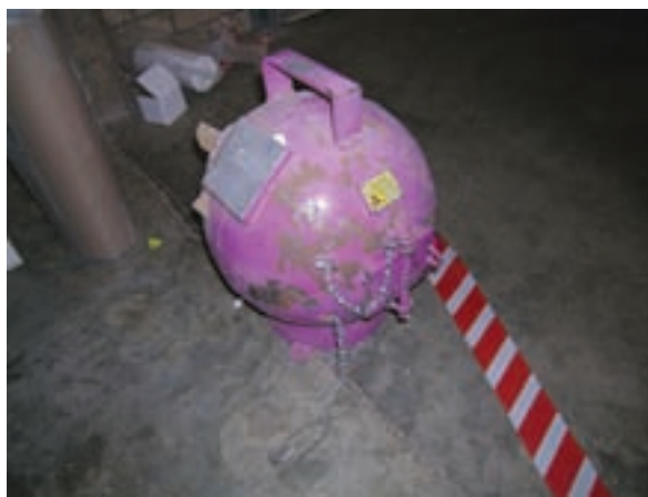
FIG. 42. Typical neutron oil well logging source transport and storage container.
