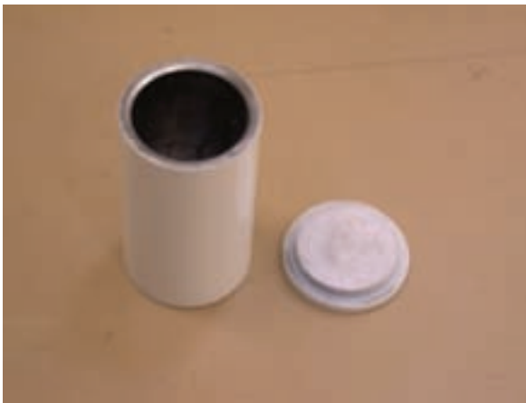
FIG. 147. Detail of an inner lead shielding container from a typical single use Type A source package (see Fig. 146) (photograph: QSA-Global).
