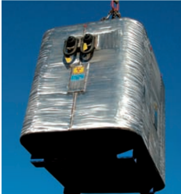
FIG. 17. Blood irradiator shielded cavity overpack for transport (photograph: MDS Nordion).
