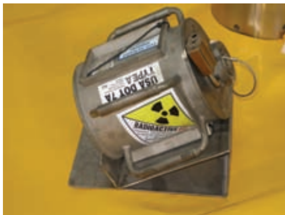
FIG. 35. Typical ^{137}\text{Cs} oil well logging source carrying shield (transport container), 37 kg \times 170 mm diameter \times 210 mm length (photograph: Schlumberger).
