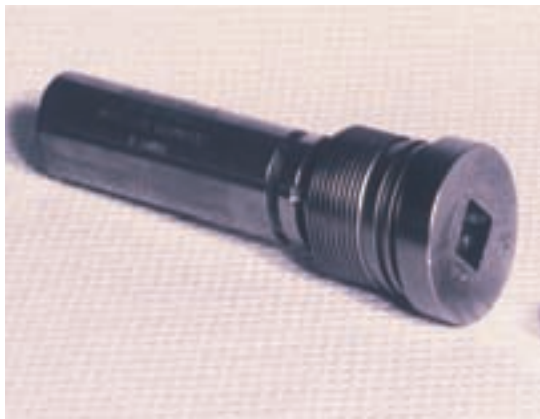
FIG. 115. Typical ^{241}\text{Am}/\text{Be} oil well logging source attached to a bull plug device (photograph: NRC).
