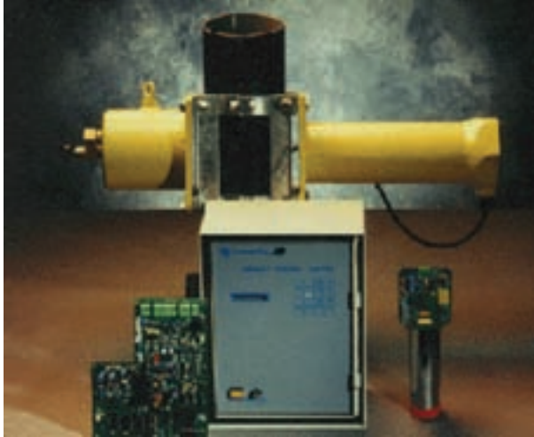
FIG. 64. Gamma density gauge fitted to a section of tube.
