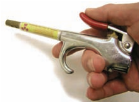
FIG. 90. Typical static eliminator air gun (photograph: Oak Ridge Associated Universities).
