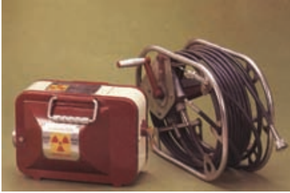
FIG. 46. Typical modern portable gamma radiography projector (photograph: BRIT).
