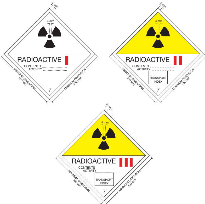
FIG. 5. Examples of the types of labels required for packages containing radioactive sources.
