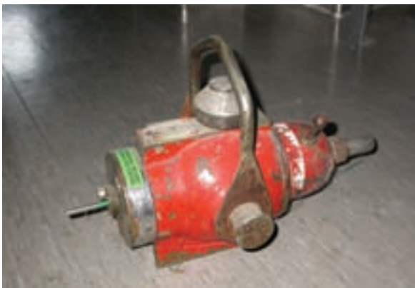
FIG. 48. Typical superseded ^{60}\text{Co} gamma radiography projector (photograph: NE-Seibersdorf).
