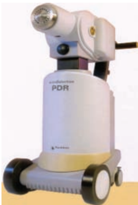
FIG. 83. Modern ^{192}\text{Ir} brachytherapy remote afterloading machine (photograph: Nucletron).
