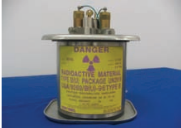
FIG. 139. Source changer ready to link to a radiography device for source exchange (photograph: QSA).
