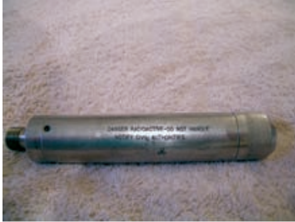
FIG. 36. Typical ^{241}\text{Am}/\text{Be} neutron oil well logging source.
