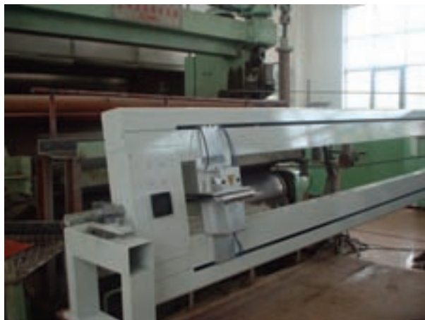
FIG. 72. Beta gauge in place on a web processing mill (photograph: Betarem).
