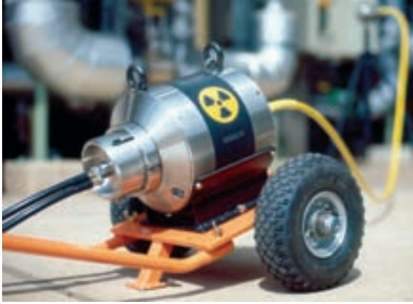
FIG. 53. Typical modern semi-portable ^{60}\text{Co} gamma radiography device (photograph: MDS Nordion).
