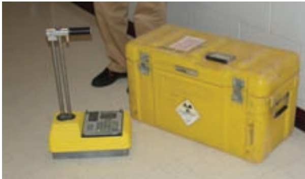
FIG. 77. Typical soil moisture and density gauge, shown with a carrying case (photograph: Troxler Labs).
