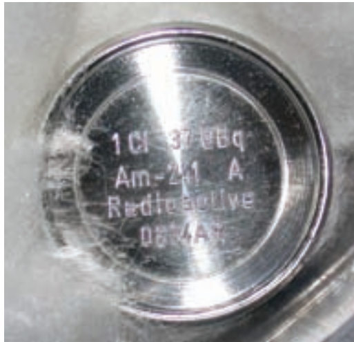
FIG. 119. Large area ^{241}\text{Am} low energy gamma source showing a welded face (approximately 40 mm diameter) (photograph: QSA-Global).
