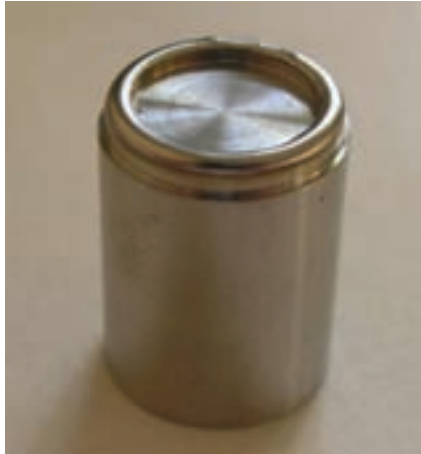
FIG. 113. Typical ^{241}\text{Am}/\text{Be} neutron source (photograph: MAYAK P.A.).
