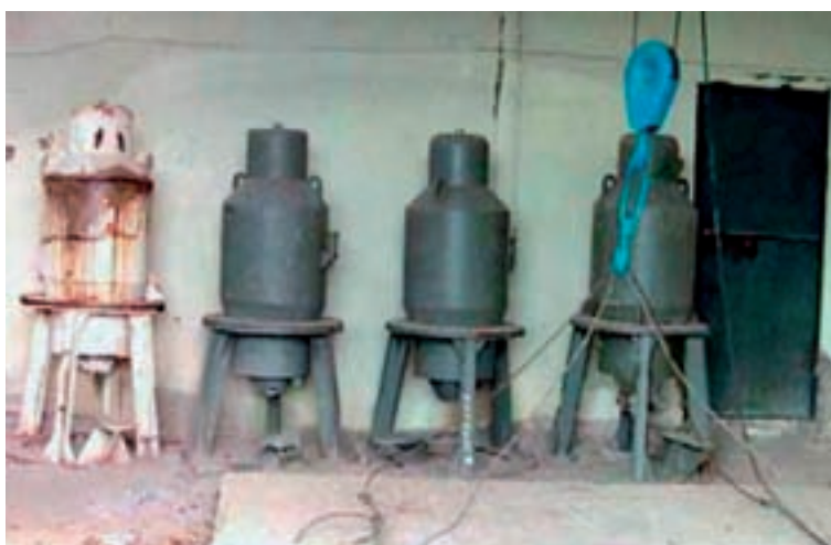
FIG. 26. Mobile caesium irradiators in the former Soviet Union containing 3500 Ci of caesium.
