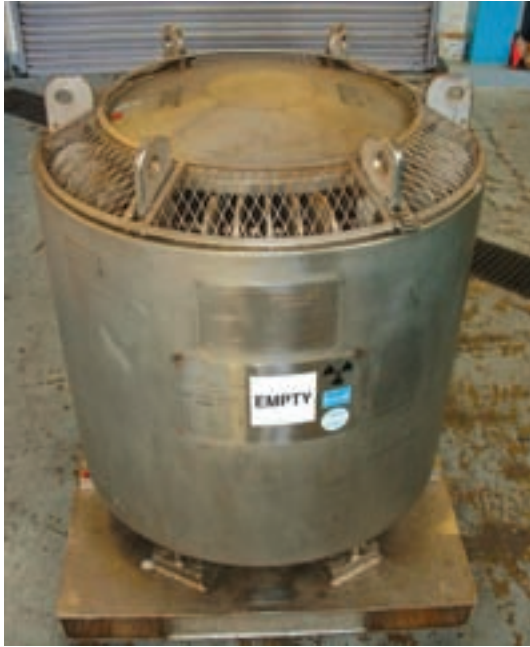
FIG. 134. High activity gamma source container in a transport configuration (photograph: REVISS).
