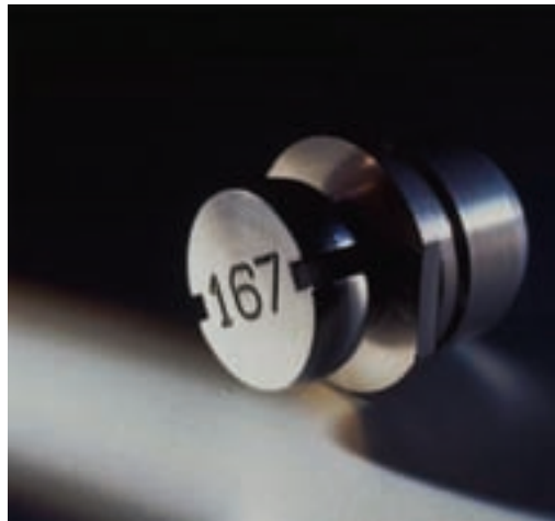
FIG. 100. Gamma knife source capsule (photograph: Elekta).
