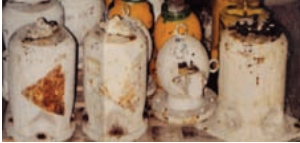
FIG. 62. Various decommissioned gamma gauge source containers.
