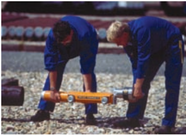
FIG. 59. Pipeline crawler being loaded into an open pipeline (photograph: MDS Nordion).
