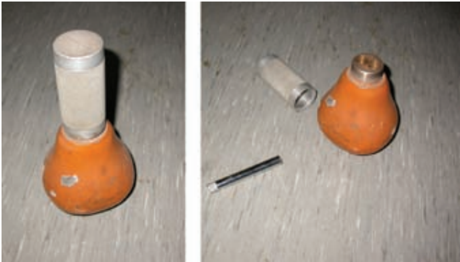
FIG. 52. Example of a superseded gamma radiography projector with manual exposure of source (photograph: NE-Seibersdorf)
