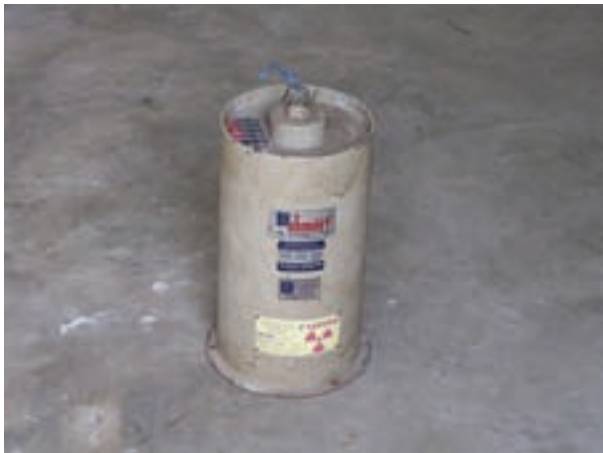
FIG. 67. Typical gamma gauge source container.
