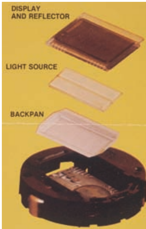
FIG. 95. Construction of a self-luminous sign.
