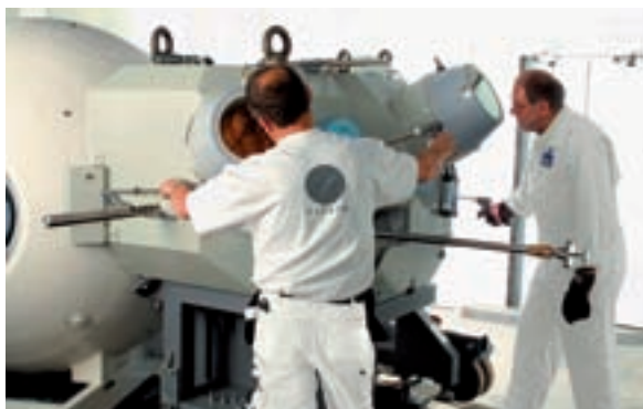
FIG. 21. Typical gamma knife reloading system (photograph: Elekta).
