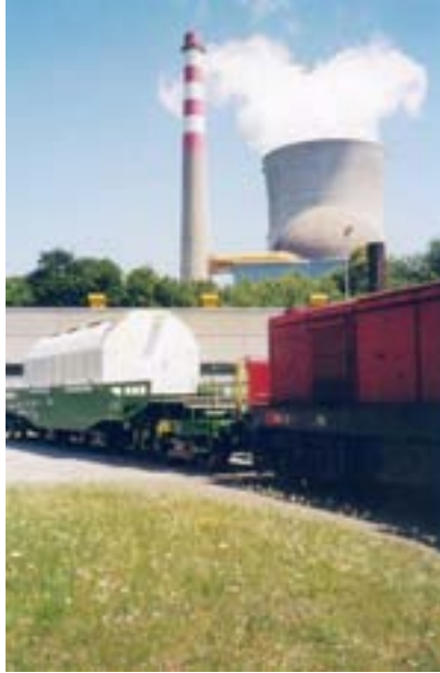
FIG. 17. Departure of spent fuel on a wagon from a nuclear power plant to be reprocessed at the La Hague facility.
