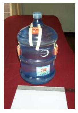
FIG. 19. Water bottle as used in lieu of human phantoms for the reconstruction of the dose.
