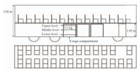
FIG. 11. Plan and elevation views of the bus in which the radiography equipment was transported.
