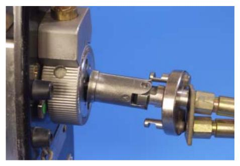
FIG. 6. The two parts of the cylindrical metal collar are closed over the connector (to the right of the connector is a disc with keyed metal lugs).
