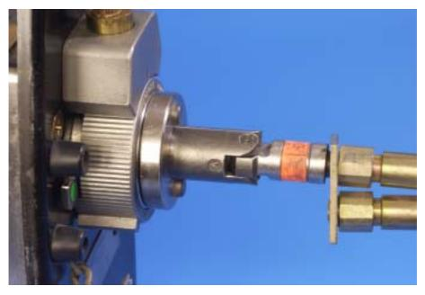
*FIG. 8. The lugs are fully engaged and the locking ring is rotated to hold the drive cable captive.*
