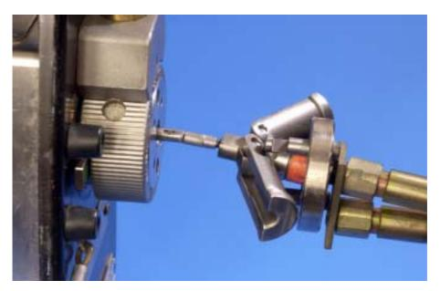
FIG. 5. Drive cable connected to the source pigtail. The two parts of the cylindrical metal collar are in the open position.
