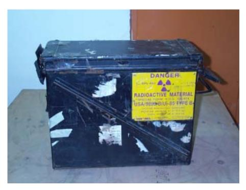
FIG. 9. Overpack for the source container.
