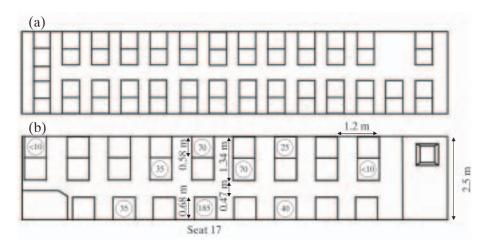
FIG. 20. Doses (mGy) registered by the dosimeters distributed on the bus seats during the dose reconstruction. Plan views of (a) the bus involved in the accident and (b) the bus used in the dose reconstruction.
