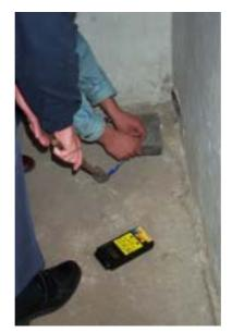
FIG. 13. Returning the source to the safe position.
