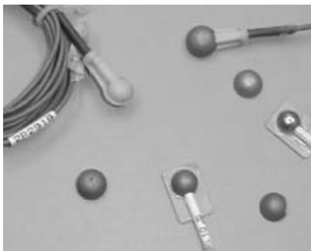
FIG. 1. Examples of diodes and brass buildup caps.
