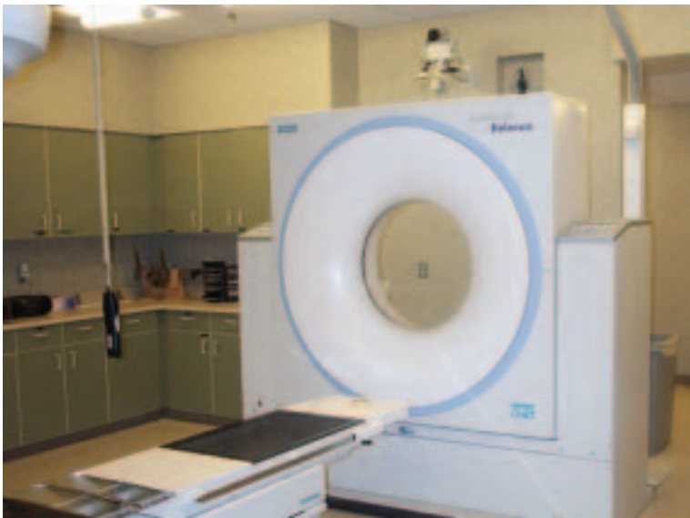
FIG. 6. The Siemens CT on rails system for IMRT target localization.
