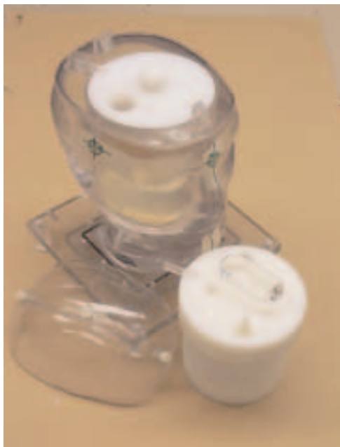
FIG. 1. The RPC's redesigned IMRT head and neck phantom with imaging insert installed. The Barex BANG gel insert is shown in the foreground.
