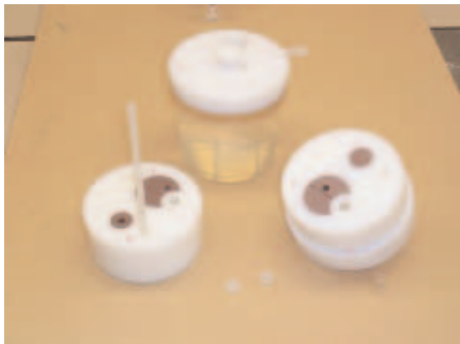
FIG. 2. The BANG gel and imaging–dosimetry inserts. Note the planning target volumes, organ at risk and film–TLD provisions in the disassembled imaging insert.
