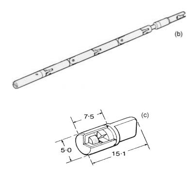
FIG. 1. (a) Gamma projector, (b) source holder, and (c) source. The size of the source is given in mm.
