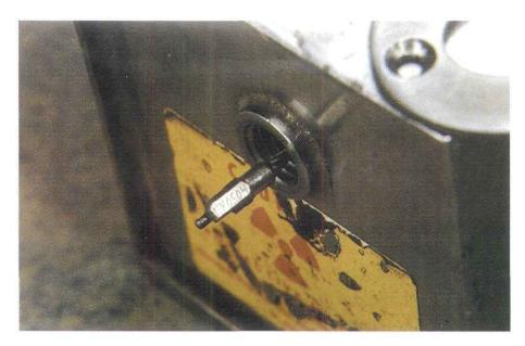
Photo 1. Source pigtail ready for connecting to drive cable.
