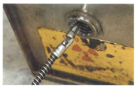
Photo 2. Source pigtail connected to drive cable.
