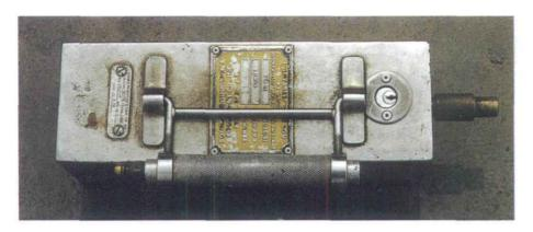
Photo 3. Radiography camera showing labels and lock.
