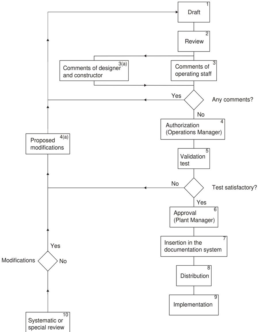
FIG. II.1. Flow diagram for the development of operating procedures.
