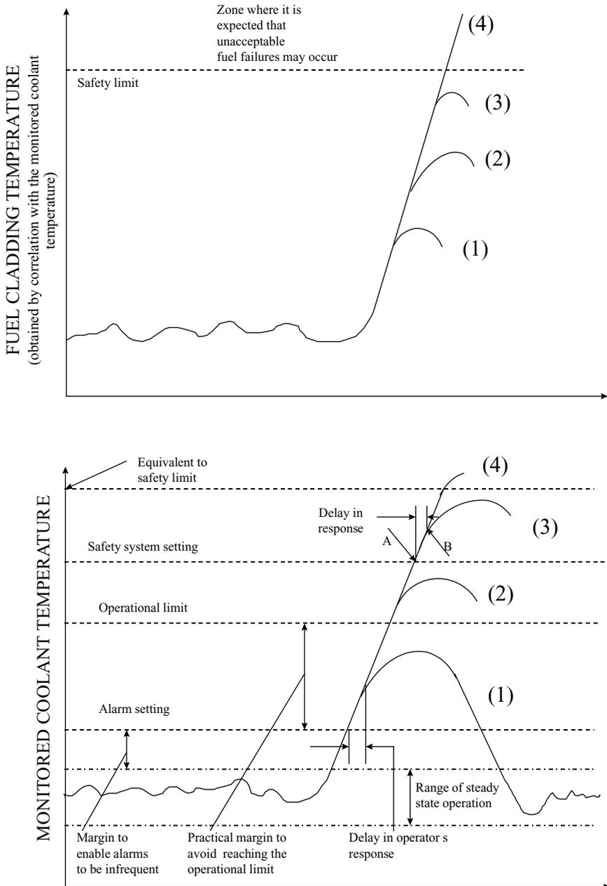
FIG. A-1. Interrelationship between a safety limit, a safety system setting and an operational limit.
