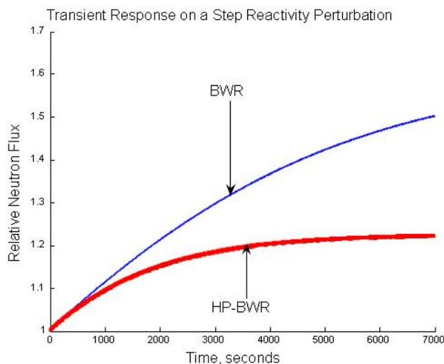
*Fig. 7. Long term stability without the use of any control system calculated with the MATLAB code (inherently stable reactor)*
