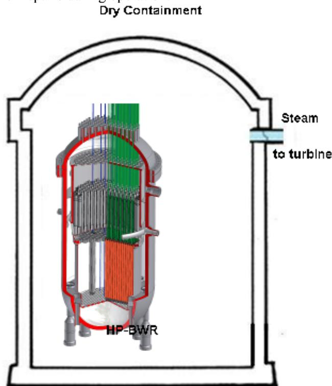
*Fig. 8. HP-BWR in a dry containment*
