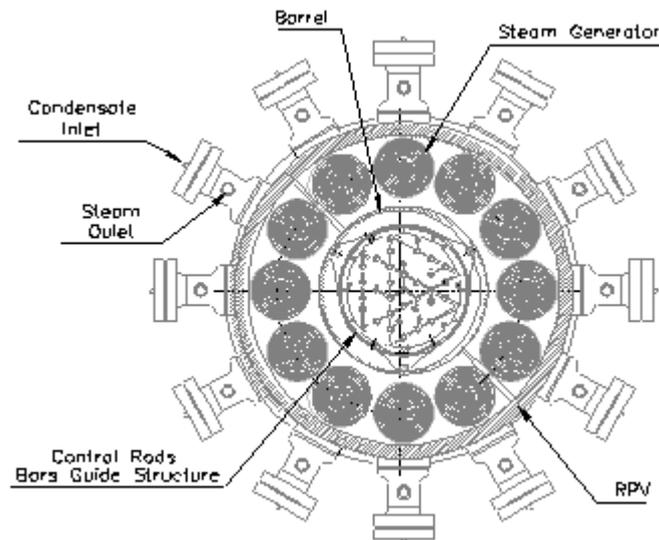
*Fig. 4. Steam Generation lay out*
