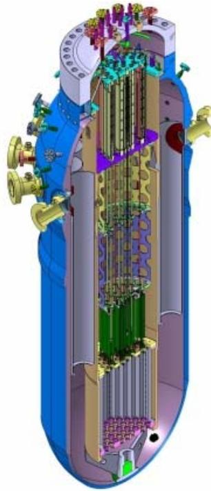
*Fig. 1. Reactor Pressure Vessel*
