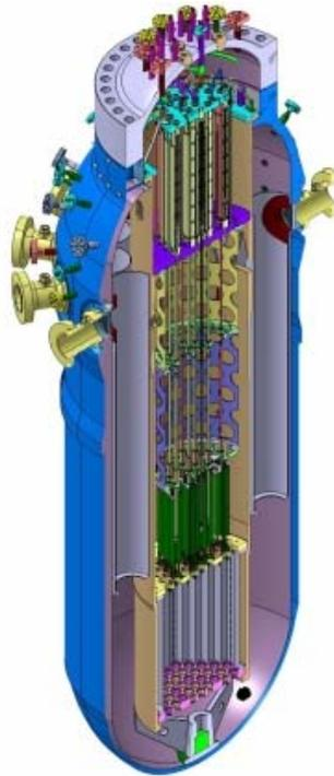
*Fig. 1. Reactor Pressure Vessel*
