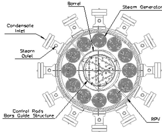
*Fig. 4. Steam Generation lay out*
