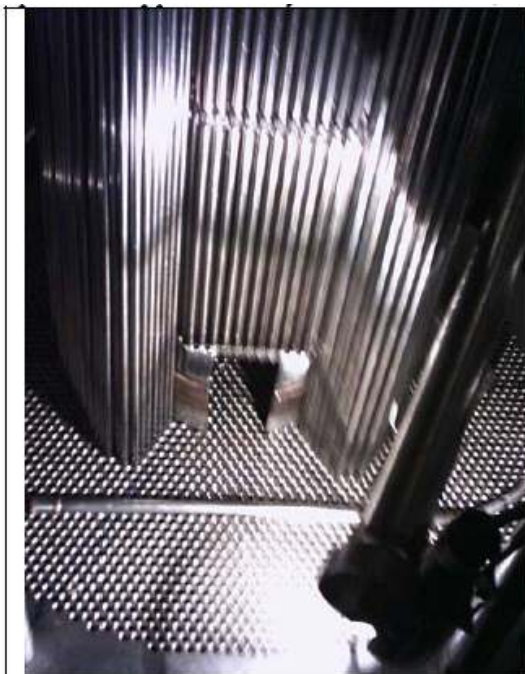
Fig. 1. The bottom of core (fuel rods of peripheral part are taken from sector of symmetry 60 deg.).
