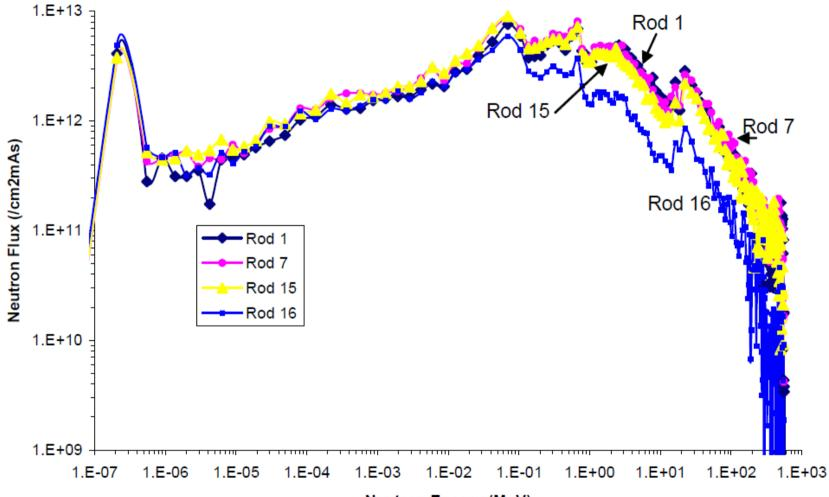
Neutron Spectrum at the Segment (-0.5-0.0 cm) of Central and Side Rods
