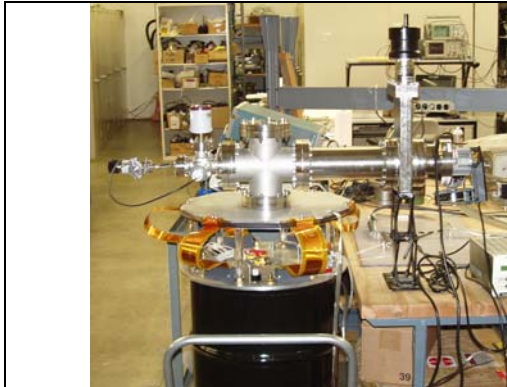
Figure 1: Photograph of 3:1 step-down unit module Thyatron/transformer driver
