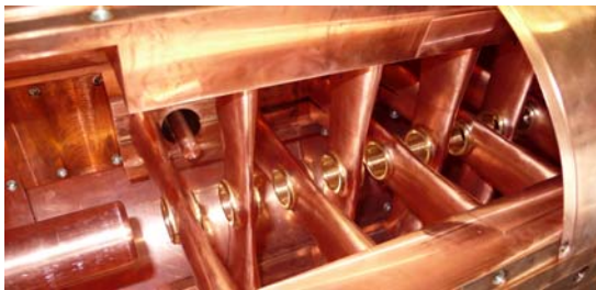
FIG. 9. Photograph of the rt copper model to validate electrodynamic simulations (left), manufacture of a girder extension aligned to the length of the first EUROTRANS CH-cavity (right).
