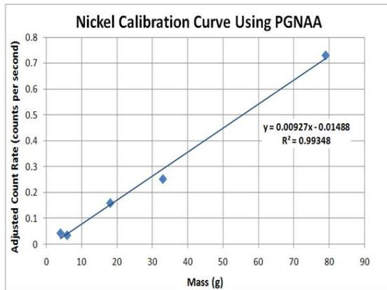
FIG. 7. Calibration curve for pure Nickel. The count rate has been adjusted to account for sample physical properties.
