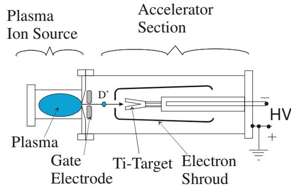
FIG.1. Simple diagram of the principle components of the neutron generator using the D-D reaction.
