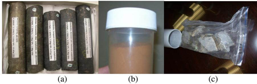
FIG. 6. Examples of mining samples tested in Heliocentric's prototype Elemental Analyzer. Split rock samples (a), Powder (b) and "lump samples" (c).
