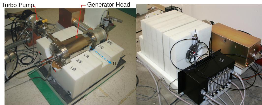
FIG. 2. The model DD-109 neutron generator head shielded inside a polyethylene housing.
