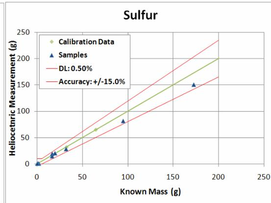
FIG. 8. A graph comparing measured mass versus the known sample mass for sulfur in customer samples. All measurements are within +/- 15% of the actual values.
