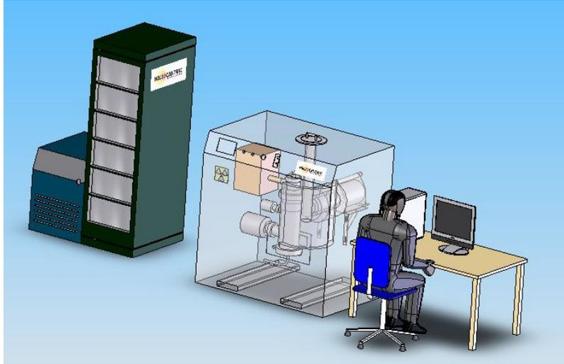
*FIG.5. Pre-Production concept of the Elemental Analyzer. The electronics rack and cooler (left), the Adelphi neutron generator, moderator/shielding and detector (center, translucent), command station and operator (right).*
