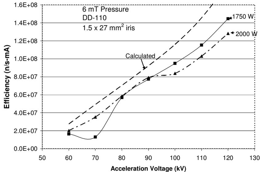
FIG. 3. The efficiency of neutron production per mA of beam current as a function of accelerator voltage for two RF plasma powers.
