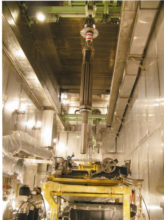
FIG. 2: The positioning of dummy target, used during the test campaigns, over the saw.
