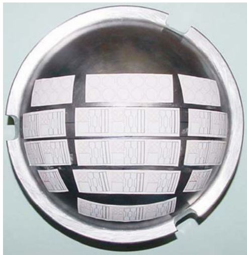
FIG. 6: Sample extraction layout for the beam entrance region of the beam entrance region of the LLMC.
