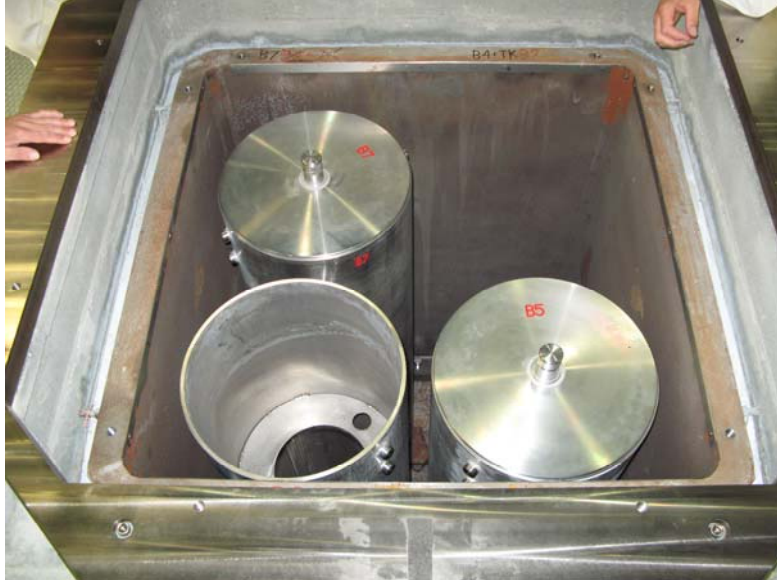
FIG. 4: The steel containers with the waste material are placed in a reinforced standard concrete waste container of PSI
